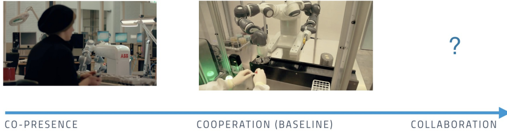
Figure 3.4: Most common examples of collaborative workspaces in industry. Co-presence: safe parallel work on different workbenches. Cooperation: sequential operation using an illuminated button. Green for robot’s turn and orange for human’s turn. By pressing the button we switch the turn. Collaboration: Only a few prototypes. Not yet exploited on a large scale in industry.
