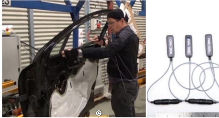
Figure 3.7: Operator wearing the Animazoo IGS120+ suit and dimension of the sensor
