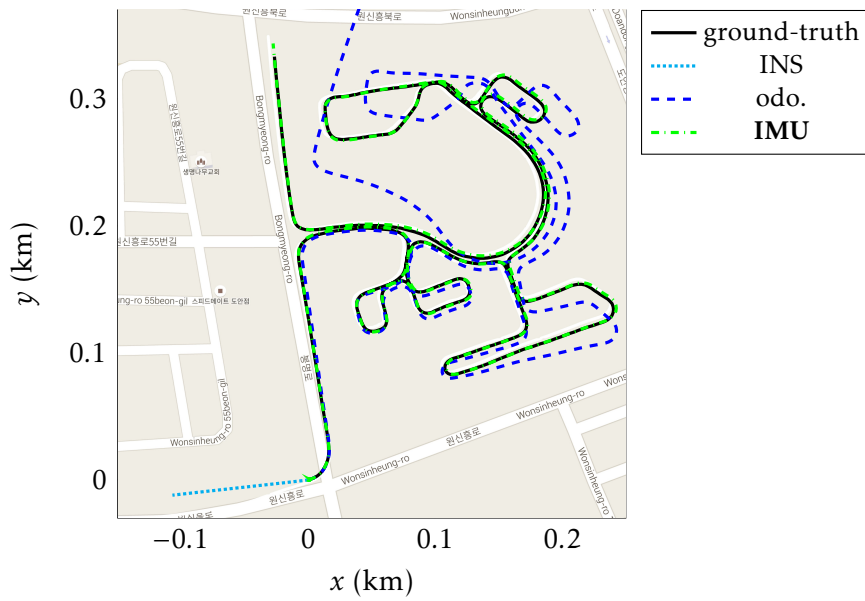
Figure 13.17: Trajectory estimates on the sequence urban07 of the KAIST dataset (2 km, 9 min). IMU is especially accurate on smooth trajectories like in this apartment complex area.
