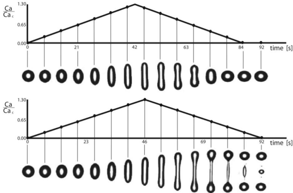
**Fig. II.5** Response of a drop under a similar triangle load of shear. All parameters are the same: maximum  $Ca/Ca_{crit} = 1.3$ ,  $p = 1.3$  but a difference of 8 s in the total duration of the experiment [Meijer et al., 2009]
