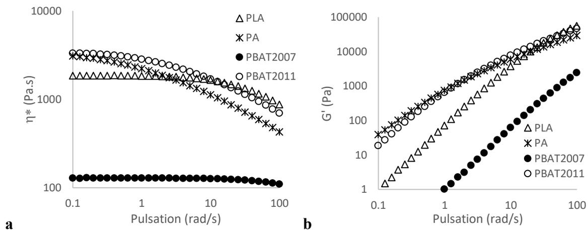
**Fig. III.1** Complex viscosity (a) and  $G'$  (b) curves for the three polymers at 180°C
