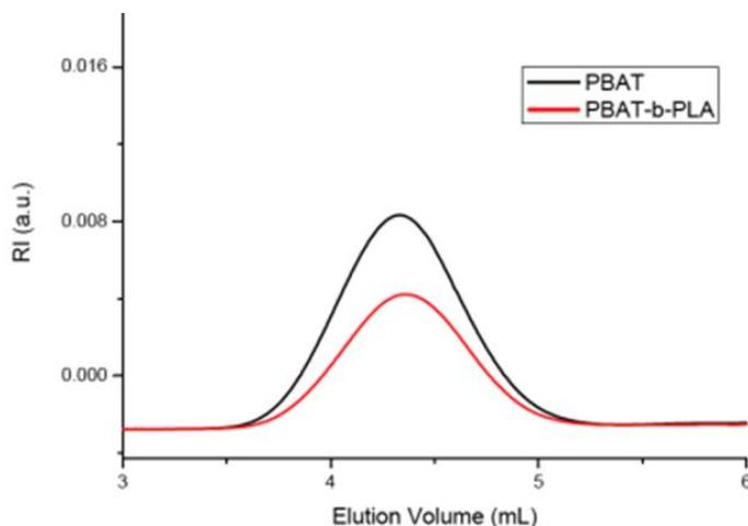
**Fig. V.11** SEC chromatograms of PBAT (black line) and PBAT-*b*-PLA (red line).
