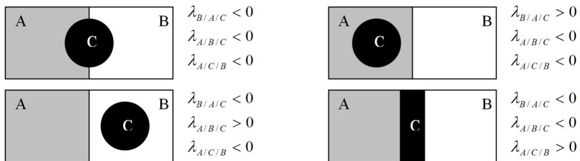
**Fig. I.1** Relation between spreading coefficients  $\lambda$  and the morphology of ternary blends composed of three polymers A, B and C.
