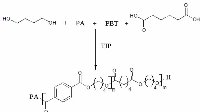
**Fig. V.9** Synthesis of PA-*b*-PBAT
