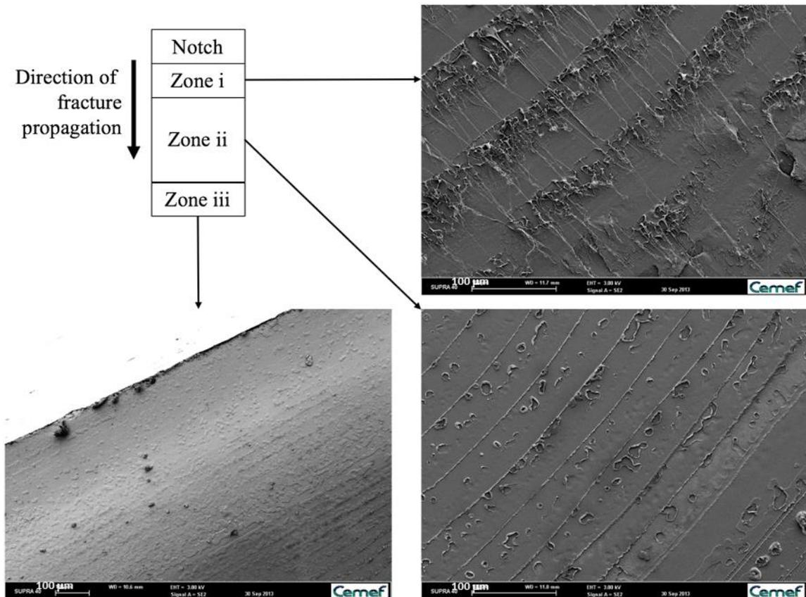
*Fig. V.34 Fracture topography of PLA after impact test*
