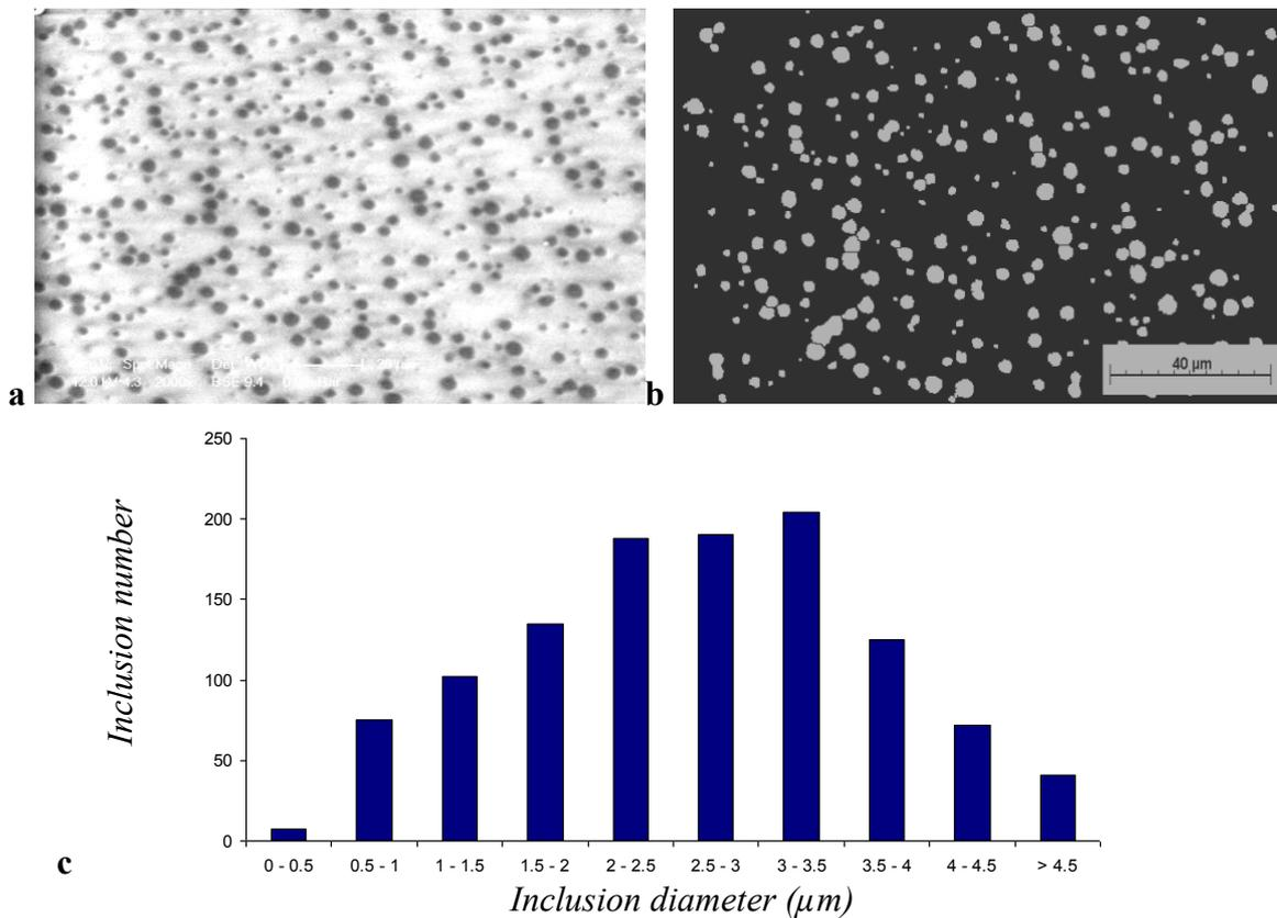
**Fig. IV.4** *a* Polished sample of 20PBAT/80PLA; *b* Treated image after binarization; *c* Size distribution of inclusions.
