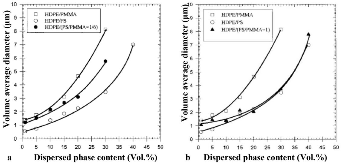
**Fig. II.13** Variation of the dispersed phase droplet size with volume ratio  $(PS+PMMA)/HDPE$  relative to the binary blends for two different volume ratios of  $PS/PMMA$ : a-  $PS/PMMA=1/6$ ; b-  $PS/PMMA=1$  [Reignier and Favis, 2000]
