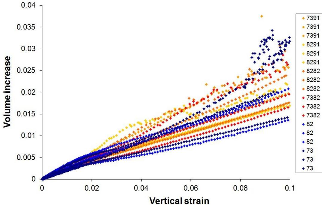
*Fig. V.33 Relationship between volume increase and vertical strain*
