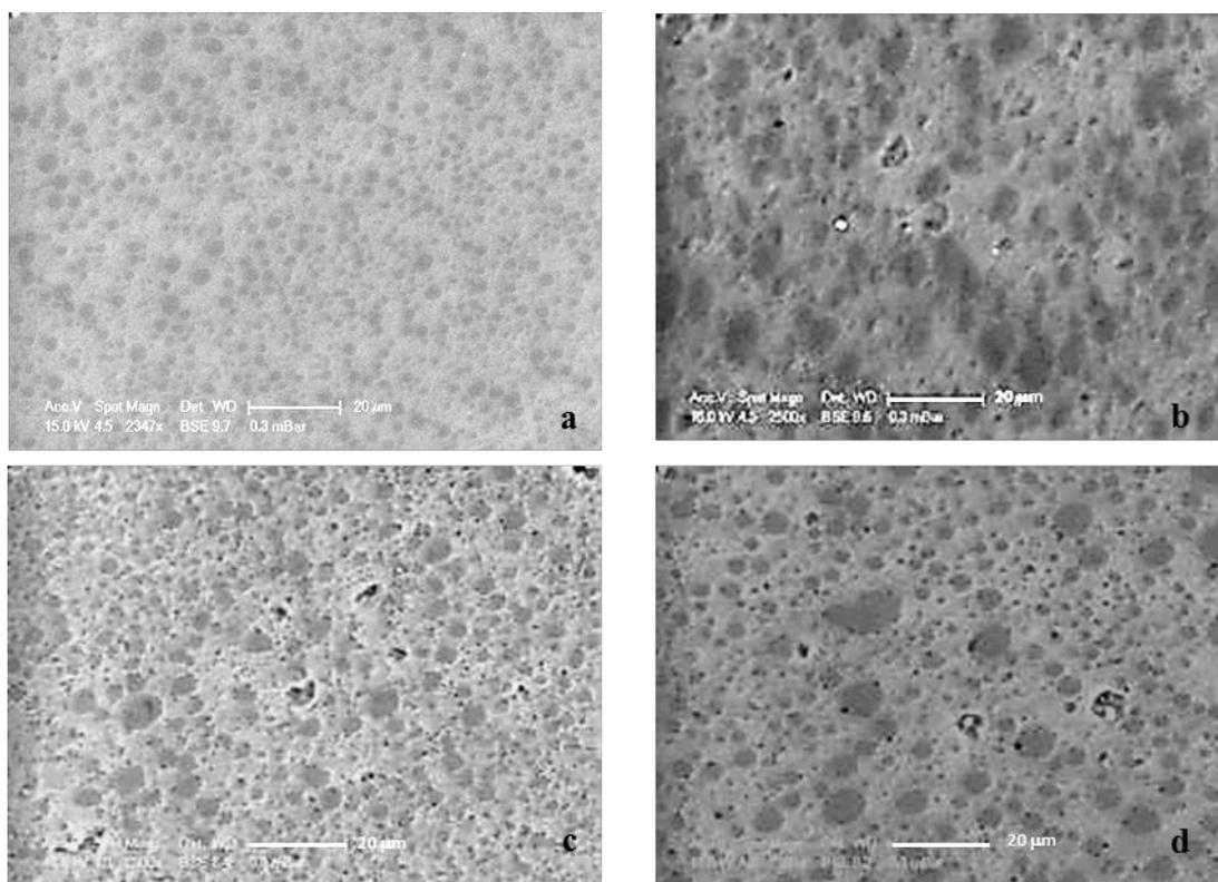
**Fig. V.3** Composition of the blends including the Lotader as compatibilizer: *a.* PLA/PBAT=65/35, *b.* PLA/PBAT/Lotader=63.4/34.2/2.4, *c.* PLA/PBAT/Lotader=61.9/33.3/4.8, *d.* PLA/PBAT/Lotader=61.9/33.3/4.8 but with a two-step order of introduction of components, at first introduction of PLA and PBAT and 3 min before the end of mixing, addition of Lotader. All blends were prepared in the micro-compounder at 50 rpm, 180 °C for 12 min
