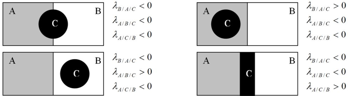
**Fig. II.11** Extension of spreading coefficient to ternary phases
