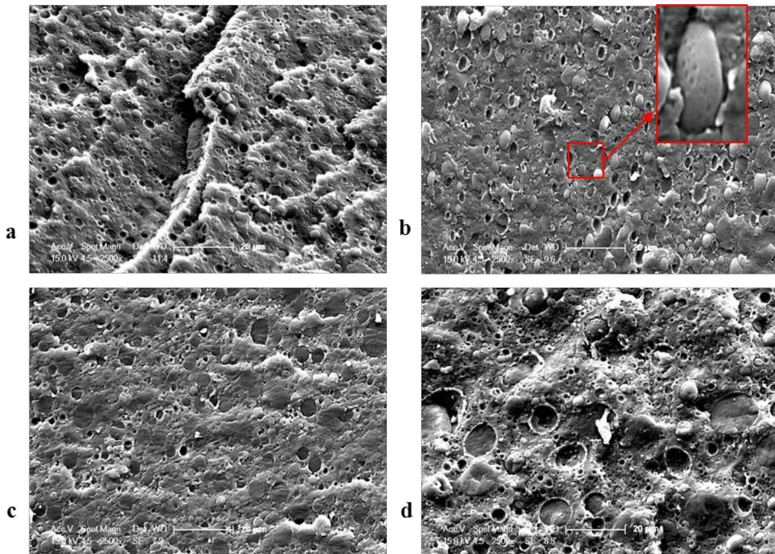
**Fig. V.4** Same samples as in Fig. V.3 prepared by cryofracture and observed by SEM: **a.** PLA/PBAT=65/35, **b.** PLA/PBAT/Lotader=63.4/34.2/2.4, **c.** PLA/PBAT/Lotader=61.9/33.3/4.8, **d.** PLA/PBAT/Lotader=63.4/34.2/2.4, with a two-step introduction - at first, introduction of PLA and PBAT, and 3 min before the end of mixing, addition of 2.4 wt% Lotader
