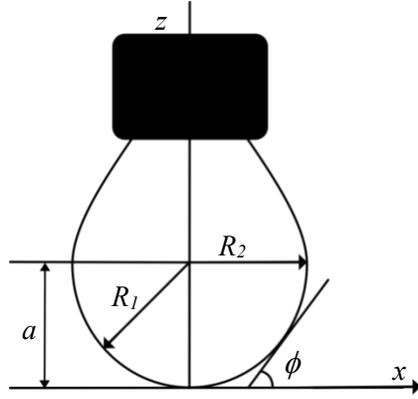
**Fig. II.15** Pendant drop geometry for an algebraic analysis
