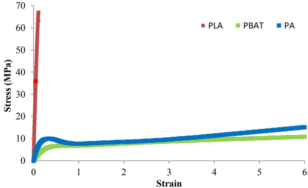
*Fig. V.27 Stress–strain curve for PLA, PBAT and PA*
