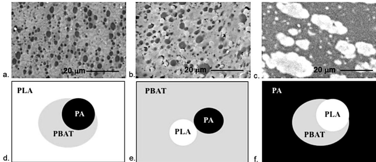
**Fig. IV.11** Morphologies of the three blends: **a** 60PLA/20PBAT(2011)/20PA; **b** 60PBAT(2011)/20PA/20PLA and **c** 60PA/20PLA/20PBAT(2011) as seen by SEM and their respective model predictions (**d** to **f**). Experimental blends were prepared in the internal mixer at 180 °C, 80 rpm for 12 min.
