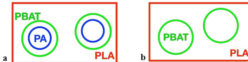
**Fig. V.20** Simplification of the ternary blend PLA/PBAT/PA (a.) into the binary blend PLA/PBAT (b.)
