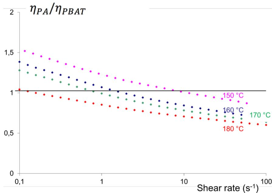
**Fig. V.23** Viscosity ratio of PA/PBAT at different temperatures
