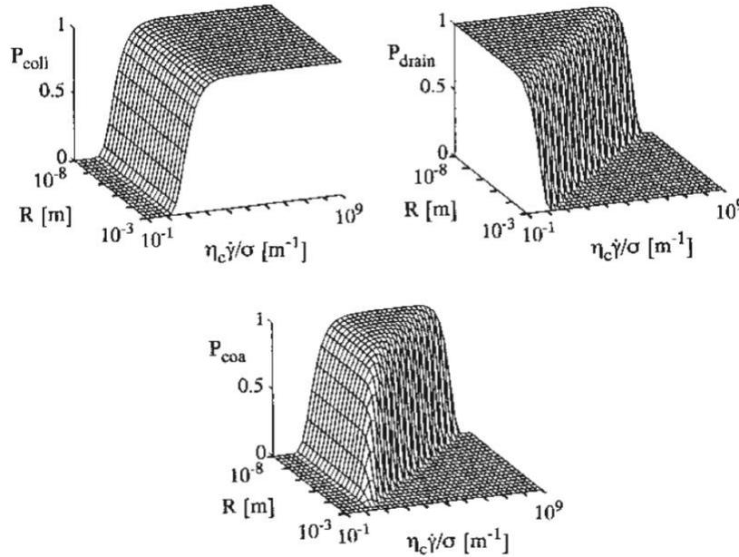
**Fig. II.6** Combination of collision and drainage probabilities under the following conditions: simple shear rate  $0.01 \text{ s}^{-1}$ ; viscosities of dispersed phase and matrix equal to  $1 \text{ Pa}\cdot\text{s}$ ;  $\gamma_{AB} = 10^{-2} \text{ N/m}$ ;  $t_{proc} = 50 \text{ s}$ ;  $h_{crit} = 10^{-9} \text{ m}$ ;  $\varphi = 0.1$ . [Meijer et al., 2009]
