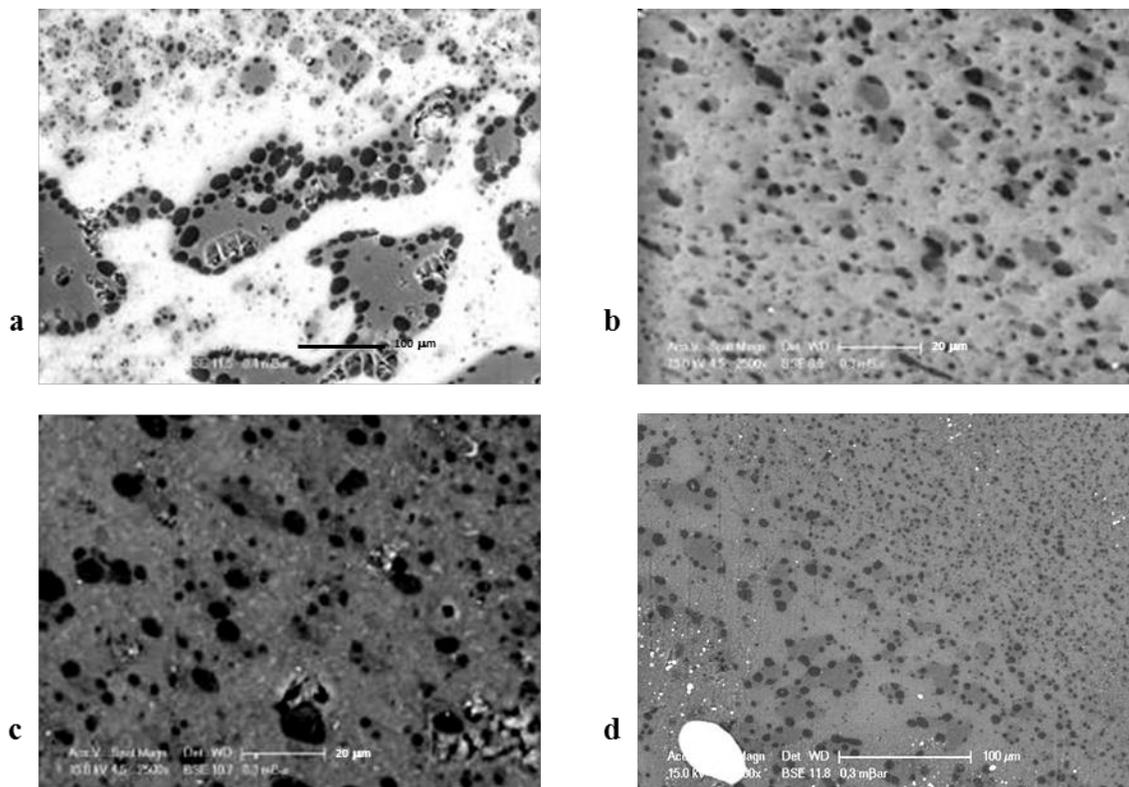
**Fig. V.5 Ternary blends including Lotader phase.** All blends prepared in the micro-compounder at 50 rpm, 180 °C for 12 min. **a.** PLA/PBAT/PA=60/27/13; **b.** first blending of PLA/PBAT/Lotader=63.4/24.2/2.4 and introduction of 13% PA 3 min before the end of mixing; **c.** first blending of 60% PLA, 24% PBAT and 2% Lotader, introduction of 13%
