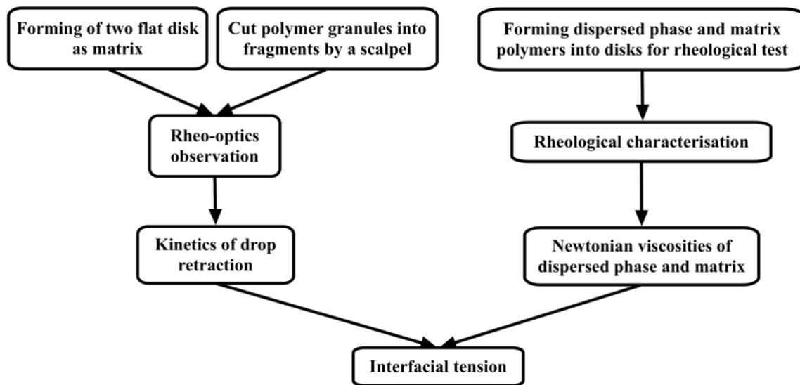
*Fig. IV.6 Working flow chart for drop retraction*
