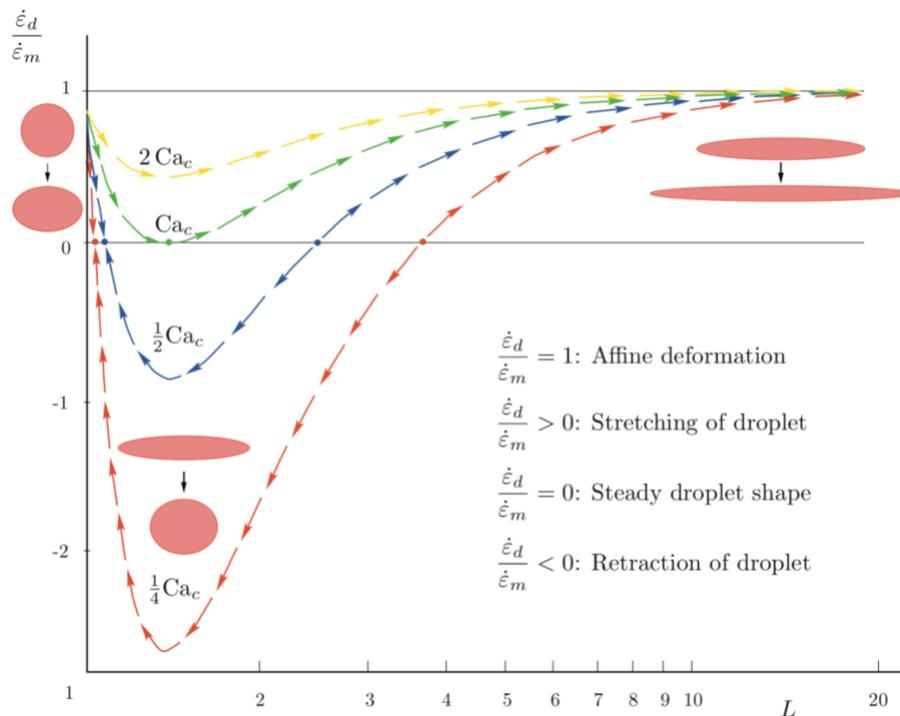
**Fig. II.4** *Dependence of the drop deformation in shear on the initial drop deformation [Stegeman et al., 2002].  $L$  represents the ratio of the length of the major axis of the deformed drop on its original radius*
