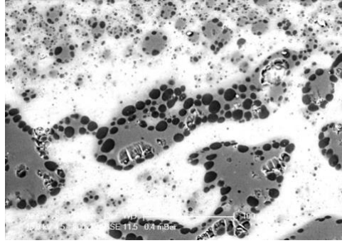
Fig. I.2 Morphology of the ternary blend 60PLA/20PBAT/20PA prepared by melt mixing. The white matrix is PLA, the grey phase is PBAT and the black phase is PA.
