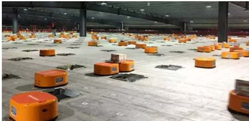
Figure 46. Self-organising and self-charging package sorting system
