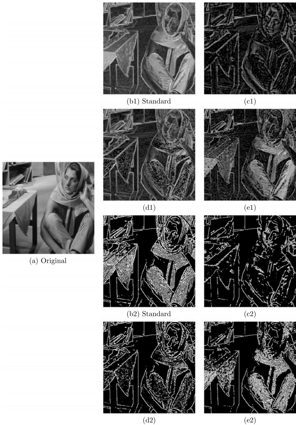
**Fig. 9** Comparative example of morphological edge detection ((\*-1) corresponds to the gradient and (\*-2) to the thresholded zero-crossing of laplacian, see the text for details): (a) original image  $f$ , (b-\*) standard transformation, (c-\*)  $(\Omega_2^{\pi/2}, \tau_{B_C}^+)$ -complex dilation
