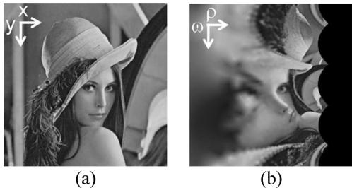
Fig. 1. (a) → (b): Example of log-pol conversion  $f(\eta) \rightarrow f(\hat{\eta})$ , where  $\eta_c$  corresponds to the center of the image, near Lena's left eye.
