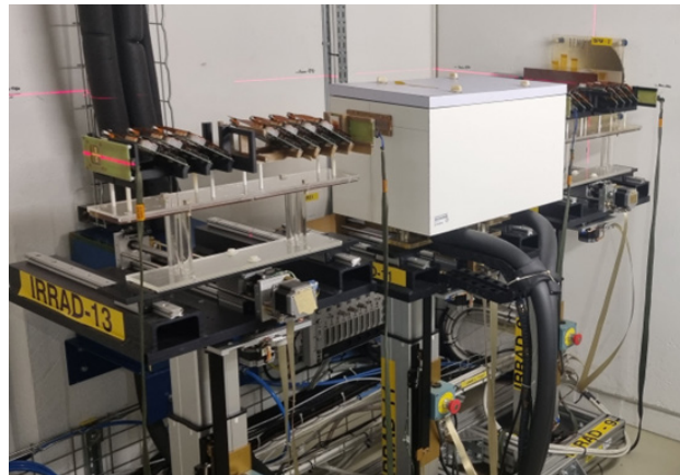
Figure 3: The three tables of IRRAD Zone 2 loaded with samples. The central table hosts a cold box.
