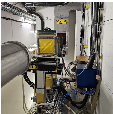
Figure 2: The protons from the PS T8 beamline exit the beam pipe on the left of the picture, transit rightward through the MWPC (in yellow) before reaching the IRRAD motorized shuttle for DUT management, near the back wall.
