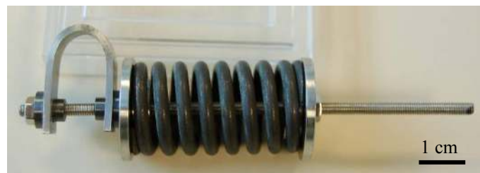
Figure 3: Photography of a U-bend specimen
