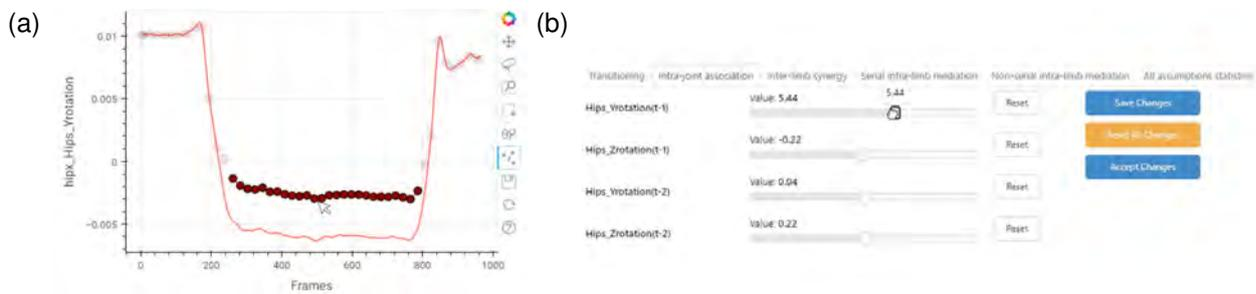
Fig. 5. Illustration to interact and modify model's coefficients to examine their effect in human postures: (a) shows how to modify time-varying coefficients by dragging the visualized data points throughout the plot. The user can select a group of dots or change only one dot. (b) illustrates the sliders to modify constant coefficients.
