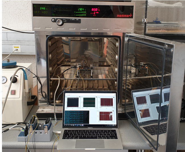
Fig. 1: Representative picture of the experimental setup. The AM572x board is inside the thermal oven. It is connected to the host system and NI cDAQ with its I/O modules NI 9215 and NI 9211. [Oven courtesy Centre des matériaux, Mines Paris, Evry]
