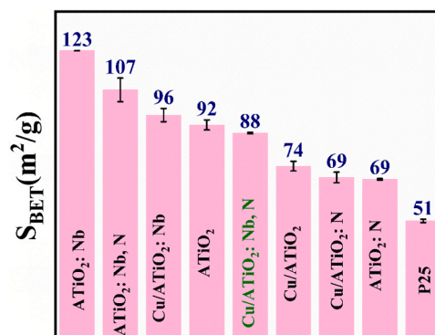
Fig. 4. Specific surface area ( S_{BET} ) of synthesized samples and commercial catalyst P25 *Instrumental error [%] = 0.6.
