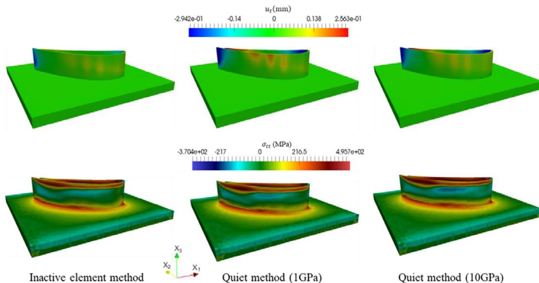
**Figure 4.** Displacement and stress distributions with inactive element method and quiet element method at the 30<sup>th</sup> layer.
