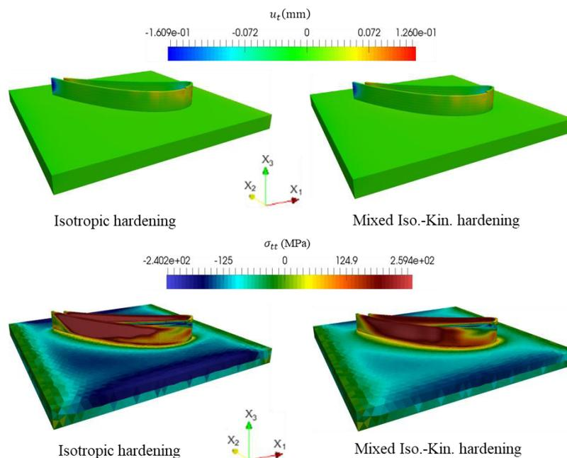
**Figure 5.** Comparison between isotropic hardening and mixed isotropic-kinematic (Mixed Iso.-Kin.) simulations: displacement field and stress field. The comparison is shown at about half the deposition of the 15<sup>th</sup> layer.
