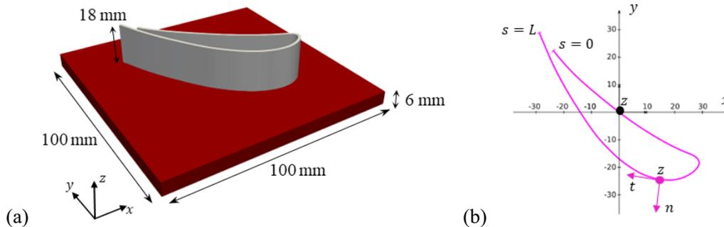
**Figure 2.** The geometry of the 30-layer turbine blade mock-up and defined coordinates: (a) 3D view; (b) deposition path in the horizontal plane, with the definition of global and local referential frames.
