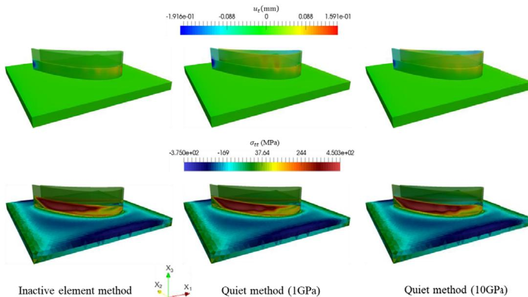
**Figure 3.** Displacement and stress distributions with inactive element method and quiet element method at the half deposition of the 15<sup>th</sup> layer. Construction domain: solid plot; non-construction domain: semi-transparent plot.
