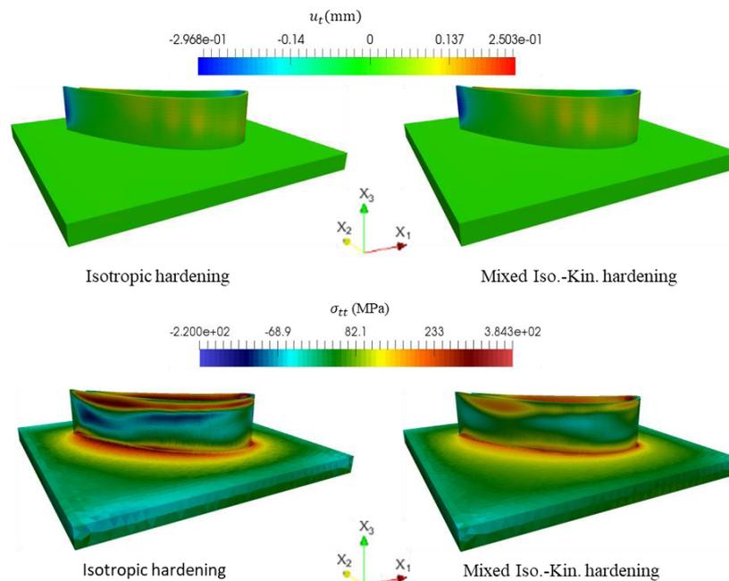
**Figure 6.** Comparison between isotropic hardening and mixed isotropic-kinematic (Mixed Iso.-Kin.) simulations: displacement field and stress field. The comparison is shown at the final deposition of the 30<sup>th</sup> layer.
