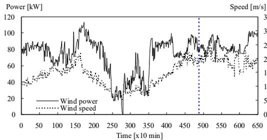
Fig. 2 : Average wind turbines power and wind speed data from the 2<sup>nd</sup> wind park of Lemnos (7x100kW).
