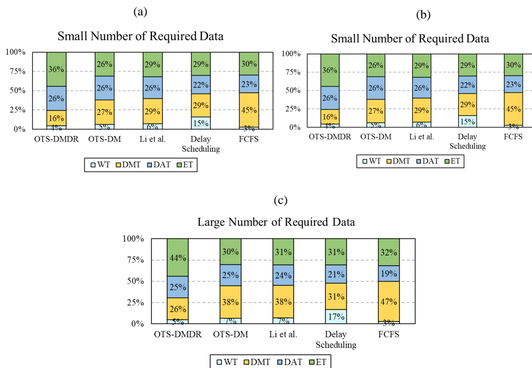
Figure 14. Percentage Response Time of Dataset Variation for the proposed methods OTS-DM and OTS-DMDR , compared to Li et al. [28], Delay Scheduling [63] and FCFS [52], where (a) is for small number of required data, (b) is for medium number of required data and (c) is for large number of required data.
