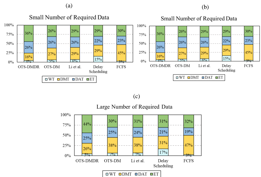
Figure 14. Percentage Response Time of Dataset Variation for the proposed methods OTS-DM and OTS-DMDR , compared to Li et al. [28], Delay Scheduling [63] and FCFS [52], where (a) is for small number of required data, (b) is for medium number of required data and (c) is for large number of required data.
