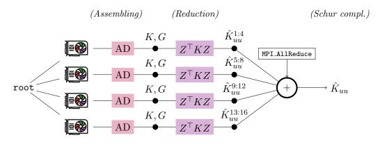
Figure 3.. Parallel computation of the Schur complement.
