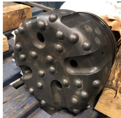
Figure 12: Drill bit designed for the test trial
