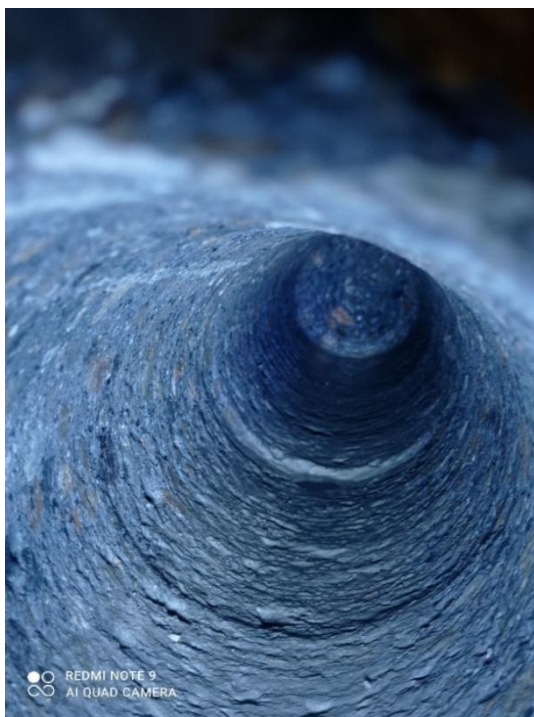
Figure 15: downhole Rotating/Sliding transition with 1° bent angle
