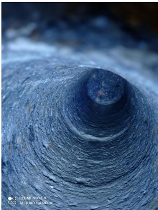
**Figure 15: downhole Rotating/Sliding transition with 1° bent angle**
