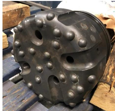
**Figure 12: Drill bit designed for the test trial**
