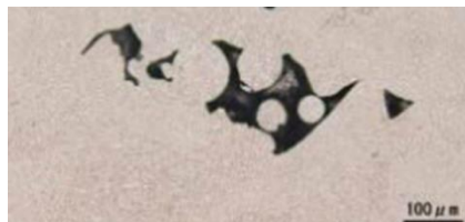
Lack of fusion, Ti-6-4, Bandyopadhyay & Traxel 18
