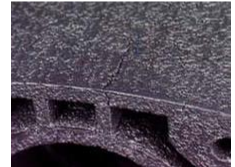
Cracks, Merzelis & Kruth 06
