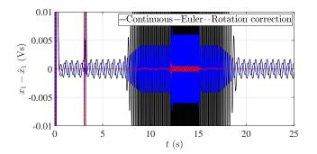
Fig. 2. Estimation error by: 1) The continuous KKL observer from [49] with  $A_c = -\operatorname{diag}(10, 44, 80)$  discretized at  $\Delta t = 0.001$  (s) (Euler); 2) The discrete KKL observer (36), (37); 3) The discrete KKL observer with rotation correction (39), (37), for  $A = e^{\Delta t A_c}$  and  $B = \begin{pmatrix} 1 & 1 & 1 \end{pmatrix}^{\top}$ .
