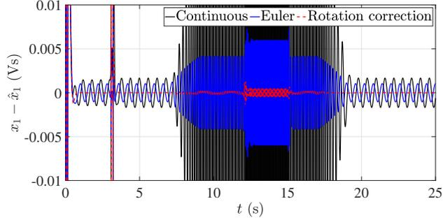
Fig. 2. Estimation error by: 1) The continuous KKL observer from [49] with  $A_e = -\text{diag}(10, 44, 80)$  discretized at  $\Delta t = 0.001$  (s) (Euler); 2) The discrete KKL observer (36), (37); 3) The discrete KKL observer with rotation correction (39), (37), for  $A = e^{\Delta t A_e}$  and  $B = \begin{pmatrix} 1 & 1 & 1 \end{pmatrix}^T$ .
