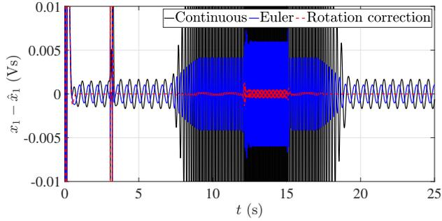
Fig. 2. Estimation error by: 1) The continuous KKL observer from [47] with  $A_c = -\text{diag}(10, 44, 80)$  discretized at  $\Delta t = 0.001$  (s) (Euler); 2) The discrete KKL observer (36), (37); 3) The discrete KKL observer with rotation correction (39), (37), for  $A = e^{\Delta t A_c}$  and  $B = \begin{pmatrix} 1 & 1 & 1 \end{pmatrix}^T$ .
