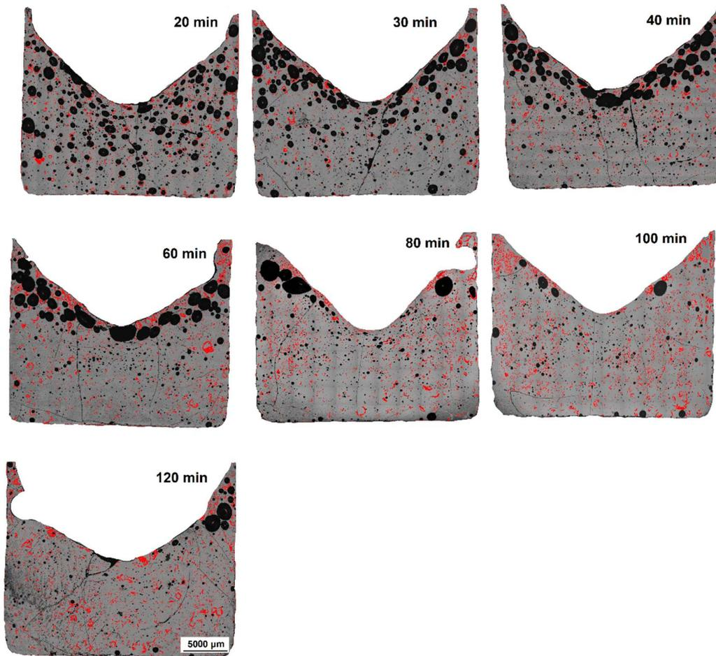
Figure 2: Optical microscope images of samples containing the borosilicate melt (grey), RuO<sub>2</sub> (red), and bubbles (black) prepared at 1000 °C for different dwell times.
