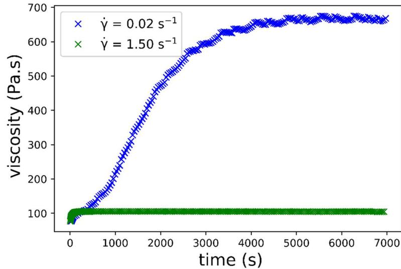
Figure 6: Viscosity measurements on the two-phase system containing the Ce-bearing borosilicate melt and RuO<sub>2</sub> crystals.
