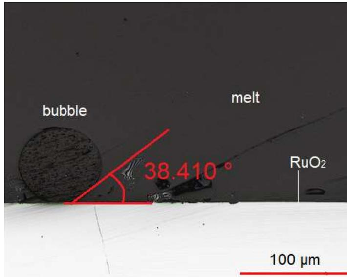
Figure S1: Example of a measurement of contact angle ( $\Psi$ ) between bubble-RuO<sub>2</sub> immersed in the borosilicate melt.
