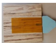
Fig. 1 : Probe orientation to measure the transversal thermal conductivity
