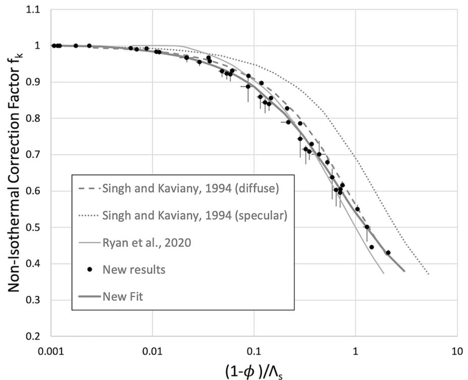
**Figure 4.** Results from simulations where particle non-isothermality was investigated. The new fit trendline is shown in addition to the trendlines from previous studies (Ryan et al., 2020; Singh & Kaviany, 1994).
