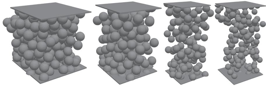
**Figure 1.** Random packing examples used in this work. The average porosity values are (left to right) 0.47, 0.60, 0.71, and 0.81. All packings are periodic in the lateral directions. The packing methods used (left to right) are Optimized Dropping and Rolling, Ballistic Deposition (single sphere), Random Sequential Packing, and Ballistic Deposition (four-sphere clusters).
