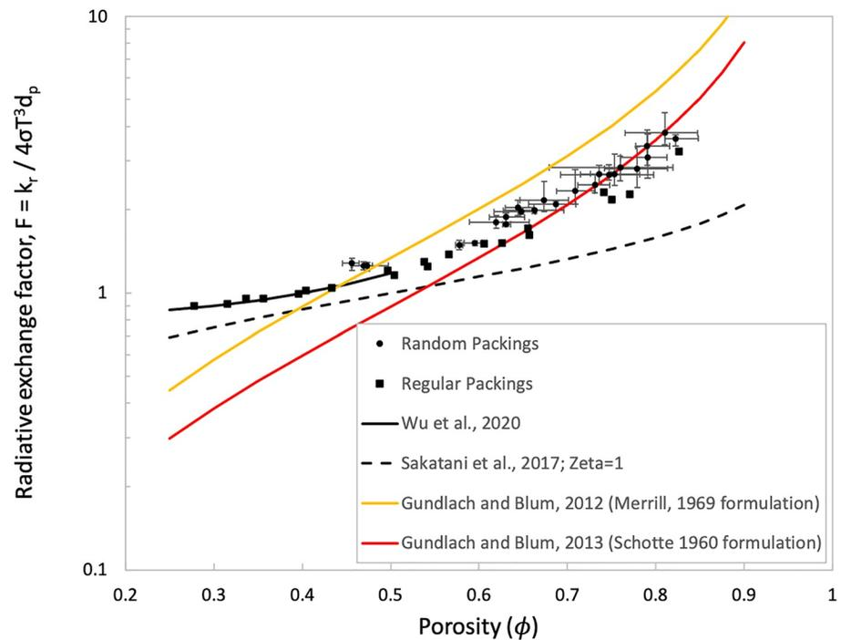
**Figure 2.** Numerical results for the radiative exchange factor as a function of porosity compared to models for regolith and sphere bed thermal conductivity. Error bars show the range of variability in porosity and  $F$  among the virtual slices within a given sphere packing geometry. The regular packings do not show error bars because there is no variability in porosity and the variability in  $F$  was smaller than the plot symbols.
