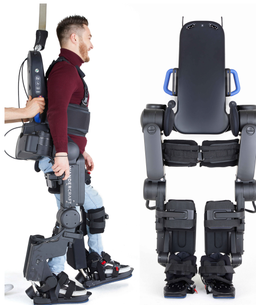
Fig. 1. A patient walks using an Atalante exoskeleton under the guidance of a physiotherapist during a rehabilitation exercise.
