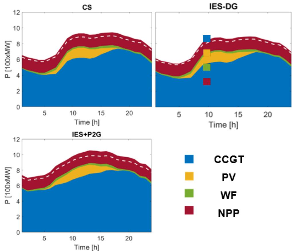
**Figure 5.**  $E_s$  and  $E_d$  for the different layouts (CS, IES-DG, IES+P2G) working in nominal conditions, when the power demand (dashed line) corresponds to Figure 4 (17 July 2018).
