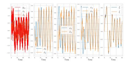
Fig. A.4. Convergence of  $(\hat{x}, \hat{\xi}) = T_a^{\text{ext}*}(z)$  to  $(x, \xi)$ , with  $(x, \xi)$  solution to (22), but where  $\dot{\xi}$  is fed with  $y_m = h(x) + \nu$  instead of y = h(x),  $\nu$  a colored white noise, z solution to (1) with input  $y_{\xi}$  and an approximate left-inverse  $T_a^{\text{ext}*}$  of  $T_a^{\text{ext}}$ . See Example 4.5 for details.
