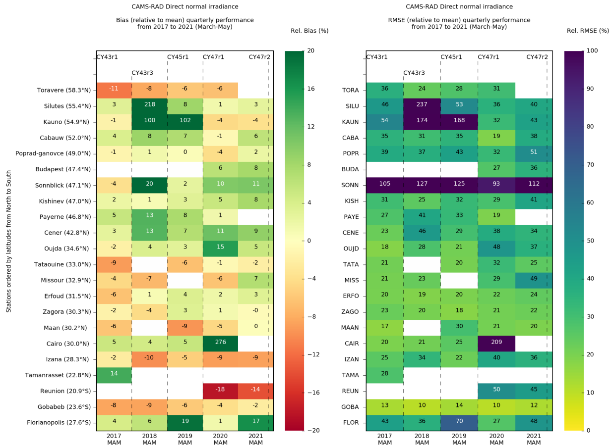
Figure 3.18b. Multi-annual direct normal irradiance relative bias (left) and RMSE (right). Top: McClear. Bottom: CAMS-RAD.
