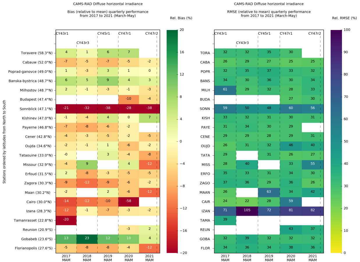
Figure 3.17b. Multi-annual diffuse horizontal relative bias (left) and RMSE (right). Top: McClear. Bottom: CAMS-RAD.
