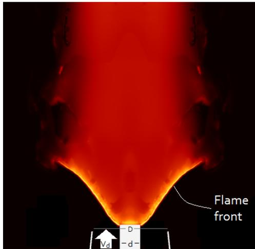
**Fig. 1** Representative view of the  $OH$  mass fraction for the steady inverted conical flame (ICF). Volume flow rate of  $\dot{V}_d = 180.3 \text{ cm}^3/\text{s}$  and fuel/air equivalence ratio  $\phi = 0.92$ .
