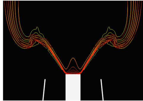
**Fig. 10** Comparison of the contour of the flame temperature for the ensemble averaged steady Fluent result (red) and the StaticROM (yellow) prediction for the ICF case 6, with a volume flow rate of  $\dot{V}_5 = 198.35 \text{ cm}^3/\text{s}$ .
