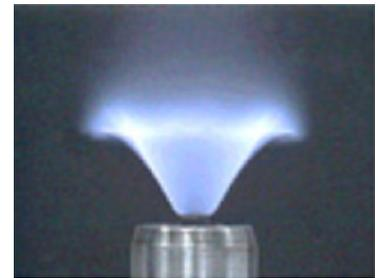
**Fig. 8 Experimental steady inverted conical flame, with equivalent ratio  $\phi = 0.92$  and nominal volume flow rate  $\dot{V}_d = 180.32 \text{ cm}^3/\text{s}$  [6].**
