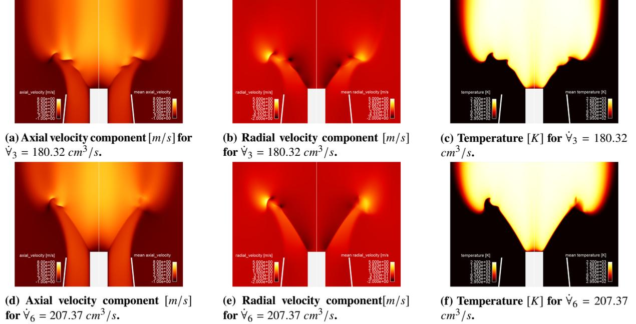
**Fig. 7 Comparison of the flame front structure between Fluent and its average: fields of velocity components and temperature, for two different fuel/air mixture flow rates. Fluent steady snapshot on the left and ensemble average on the right side.**
