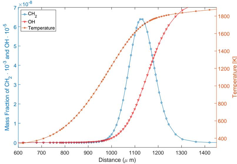
**Fig. 4** Zoom on the fields of mass fraction of  $\text{CH}_2$  and  $\text{OH}$ , and temperature ( $K$ ) obtained for the 1D freely propagating laminar premixed methane/air flame, with equivalence ratio of  $\phi = 0.92$ .
