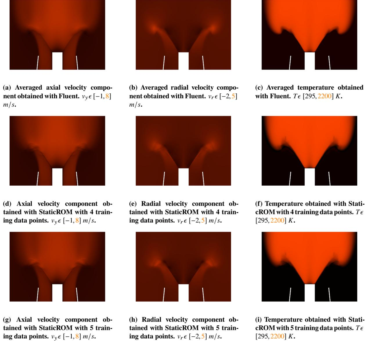
**Fig. 9** Comparison between the Fluent averaged results with ROM prediction for the averaged steady ICF, for a fuel inlet volume flow rate of  $\dot{V}_5 = 198.35 \text{ cm}^3/\text{s}$ .
