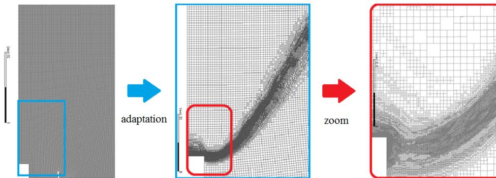
**Fig. 5** Representation of the mesh adaptation due to temperature gradient (obtained using Fluent). Left: base mesh with a size of  $100 \mu\text{m}$ ; center: mesh already adapted after the flame is developed; right: zoom on the adapted mesh.
