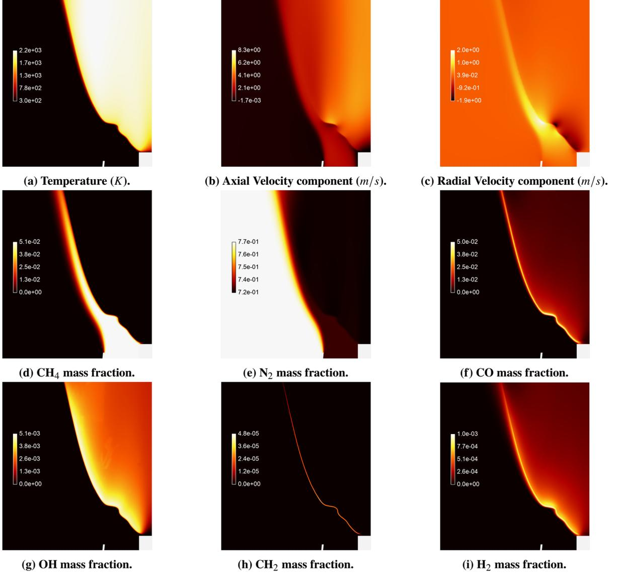
**Fig. 6** Structure of the laminar premixed inverted conical flame, with a volume flow rate of  $\dot{V}_d = 180.3 \text{ cm}^3/\text{s}$  and a methane/air equivalence ratio of  $\phi = 0.92$ .
