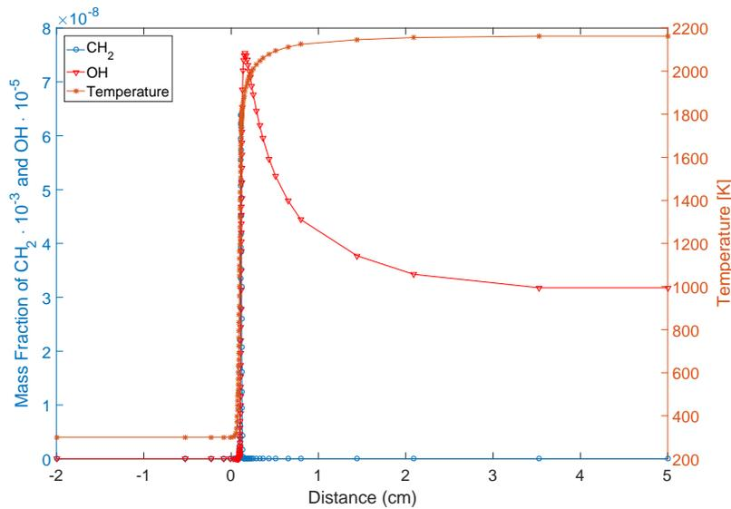
**Fig. 3** Fields of mass fraction of  $CH_2$  and  $OH$ , and temperature ( $K$ ) obtained for the 1D freely propagating laminar premixed methane/air flame, with equivalence ratio of  $\phi = 0.92$ .
