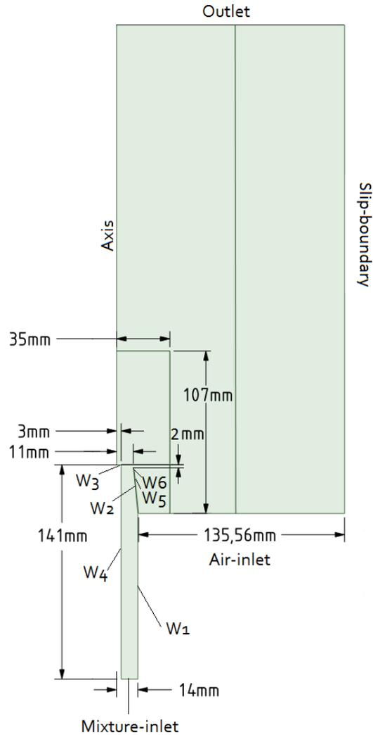
**Fig. 2** Computational domain with corresponding dimensions and boundary conditions.
