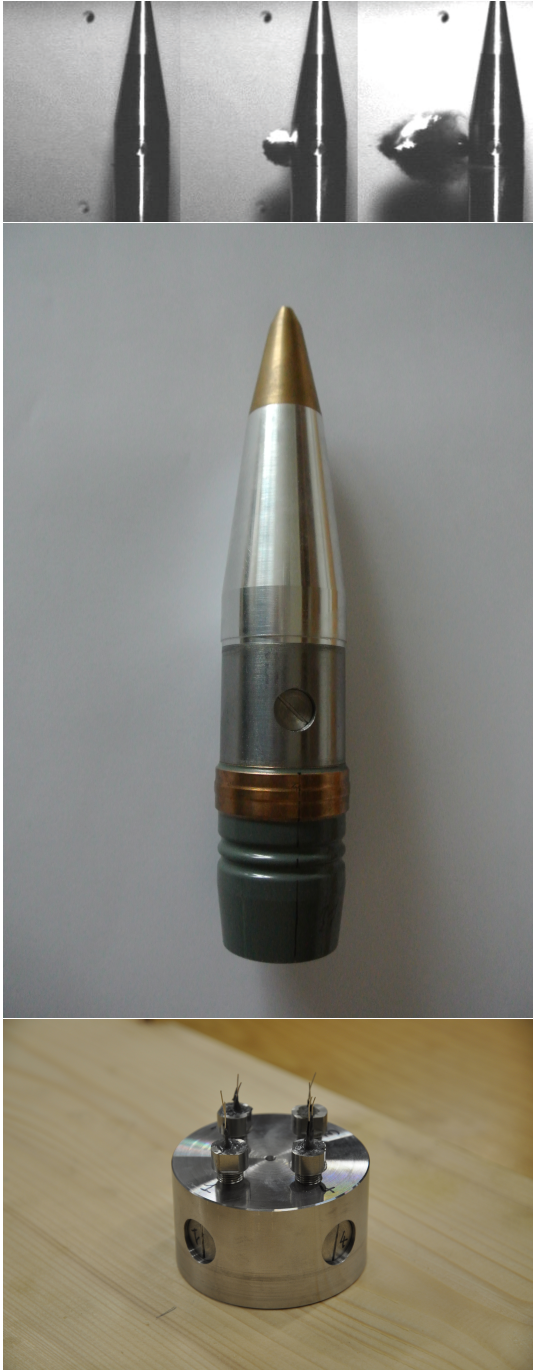
Figure 3: ISL pyrotechnical thruster. Top: close-up view during thrust. Middle: integration in a 155 mm shell. Bottom: the thruster.
