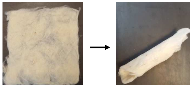
Fig. 8. Photographs of a thin kapok-based composite aerogel sheet (sample 80CA-0.096 with dimensions close to 9 cm x 9 cm x 0.2 cm, unfolded and rolled, respectively).
