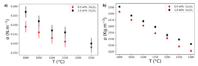
Figure 1: High-temperature results of a) surface tension between an oxygen bubble and the borosilicate melts with 0.0 and 1.0 wt% of  $Ce_2O_3$ .and b) density of borosilicate melts with 0.0 and 1.0 wt% of  $Ce_2O_3$ .
