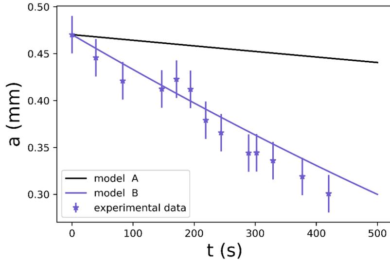
Figure 2: Bubble radius ( $a$ ) as a function of time obtained experimentally and by two numerical models: A and B. The former does not consider redox reactions on the mass transfer calculations and the latter does.
