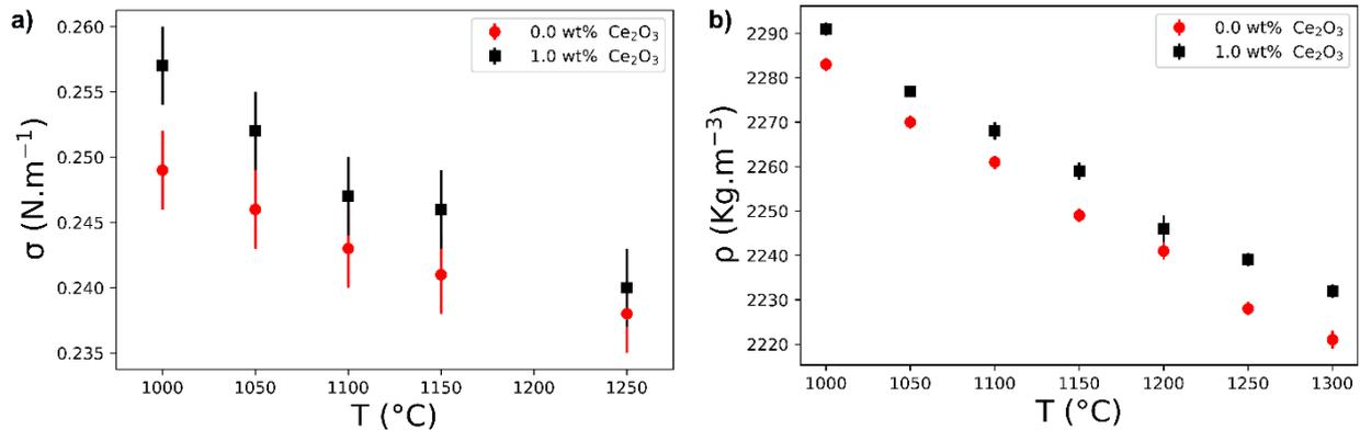
Figure 1: High-temperature results of a) surface tension between an oxygen bubble and the borosilicate melts with 0.0 and 1.0 wt% of Ce<sub>2</sub>O<sub>3</sub>, and b) density of borosilicate melts with 0.0 and 1.0 wt% of Ce<sub>2</sub>O<sub>3</sub>.
