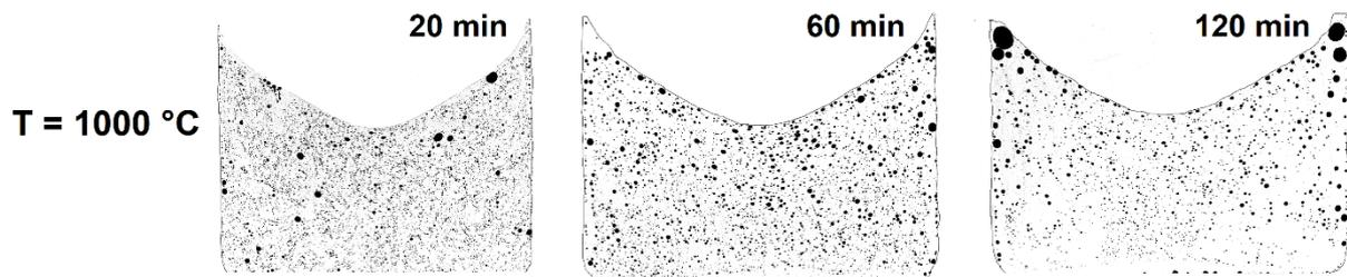
Figure 4: Binarized optical microscope images of samples treated after 1000 °C during 20, 60, and 120 min
