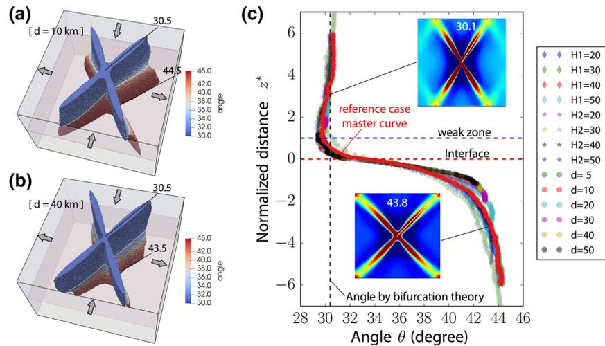
**Figure 3.** Same as Figure 2 but for nucleation in the brittle layer ( $d > 0$ ) and a reference model with  $d = 10$  km. The fault angle in the brittle layer is near-optimal and rotates toward  $45^\circ$  in the ductile layer.
