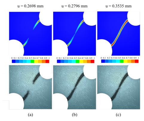
**Figure 16:** Phase field evolution at various deformation stages on the deformed configuration for a fine mesh with base element size 0.2 mm. The phase field is used to trigger the remeshing with a threshold of 0.06. The mesh topology is shown at each stage. **a**. u = 0.2698 mm. **b**. u = 0.2796 mm. **c** u = 0.3535 mm.
