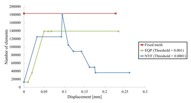
Figure 20: Evolution of number of elements for different remeshing cases along with the reference case (Fixed mesh).
