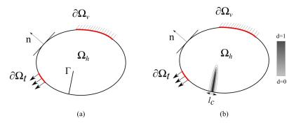
**Figure 1:** a. Geometry and boundary conditions of an arbitrary domain with discontinuity  $\Gamma$ . b. Transformation of the crack to a diffused damage with the phase field d that goes from 0 to 1.
