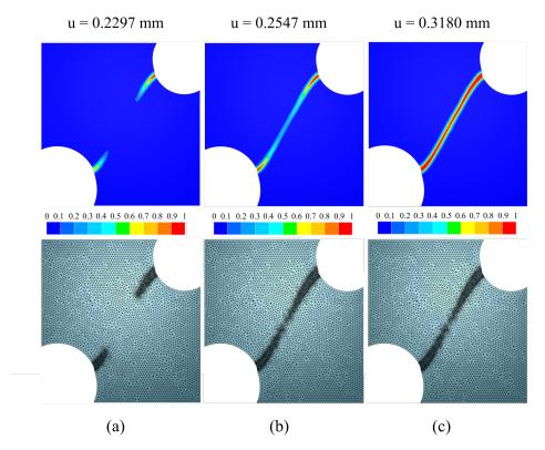
Figure 17: Phase field evolution at various deformation stages on the deformed configuration with base element size 0.15 mm. The phase field is used to trigger the remeshing with a threshold of 0.06. The mesh topology is shown at each stage.  $\mathbf{a}$ .  $\mathbf{u} = 0.2297$  mm.  $\mathbf{b}$ .  $\mathbf{u} = 0.2547$  mm.  $\mathbf{c}$ .  $\mathbf{u} = 0.3180$  mm.
