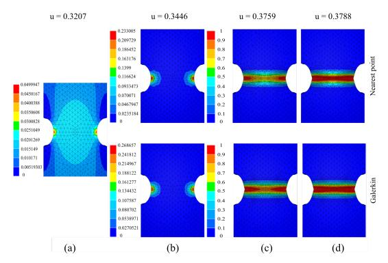
**Figure 12:** Evolution of phase field at different deformation states on the deformed configuration for a phase field threshold is set to 0.075. The average element size of the base mesh is set to 1.25 mm. **a.** u = 0.3207 mm. **b.** u = 0.3446 mm. **c.** u = 0.3759 mm. **d.** u = 0.3788 mm.
