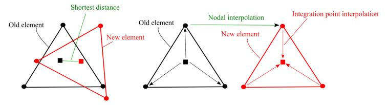
**Figure 3:** Field interpolation method: **a.** P0 transfer (Nearest point interpolation. **b.** P1 transfer with Galerkin smoothing.
