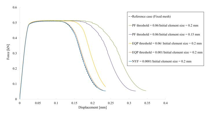
Figure 21: Force vs. Displacement curves for different remeshing cases along with the reference case (Fixed mesh). NYF is the normalized trial yield function.
