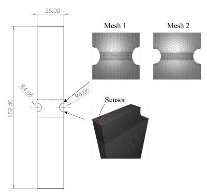
**Figure 4:** The representation of the tension test geometry and boundary conditions of a reference case [11]. The mesh is illustrated with the local refinement. The thickness of the specimen is 2.37 mm where all dimensions are in mm.
