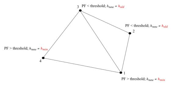
Figure 2: Calculating the new element size based on the phase field values at the nodes.
