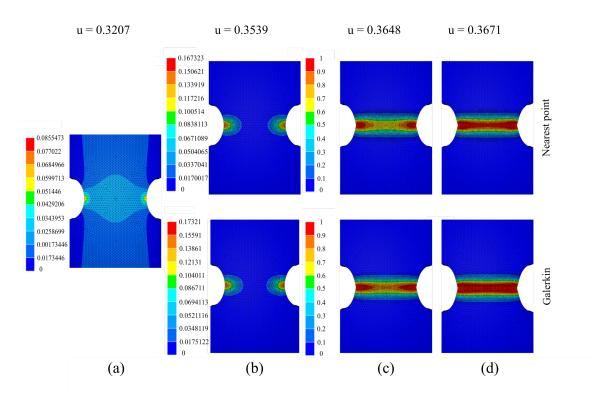
**Figure 9:** Evolution of phase field at different deformation states on the deformed configuration for a phase field threshold is set to 0.075. The average element size of the base mesh is set to 0.5 mm. **a.** u = 0.3207 mm. **b.** u = 0.3539 mm. **c.** u = 0.3648 mm. **d.** u = 0.3671 mm.
