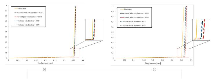
Figure 14: Comparison between the phase field evolution at a fixed mesh and with remeshing with a base element size = 0.5 mm in **a** and 1.25 mm in **b**.
