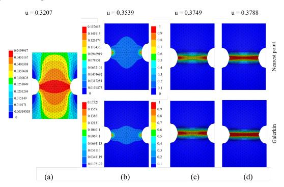
**Figure 11:** Evolution of phase field at different deformation states on the deformed configuration for a phase field threshold is set to 0.025. The average element size of the base mesh is set to 1.25 mm. **a.** u = 0.3027 mm. **b.** u = 0.3539 mm. **c.** u = 0.3749 mm. **d.** u = 0.3788 mm.
