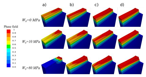
Figure 7: Contour plots of the phase field evolution for three different values for the plastic threshold  $W_0$ . Four different deformation states are illustrated starting from crack initiation at (a) until the final failure at (d).
