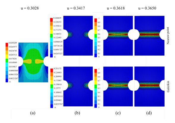
**Figure 8:** Evolution of phase field at different deformation states on the deformed configuration for a phase field threshold is set to 0.025. **a.** u = 0.3028 mm. The average element size of the base mesh is set to 0.5 mm. **b.** u = 0.3417 mm. **c.** u = 0.3618 mm. **d.** u = 0.3650 mm.
