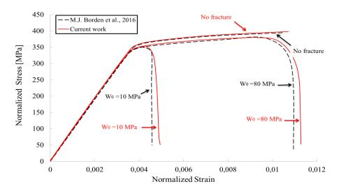
**Figure 6:** Numerical validation with the model of M.J. Borden et al. [11]. Results are reported for two different values of the plastic threshold. The time step is set to 0.5 sec during the first 125 steps in the linear regime then 0.025 sec for the rest of the simulation.
