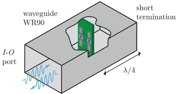
**Fig. 6 Schematic representation (not to scale) of superconducting waveguide device DTW1.** Two-qubit chip is placed  $\lambda/4$  from a short termination in the waveguide. Guided input-output waves are launched and monitored through the I-O port connecting to a standard SMA adapter (not shown).
