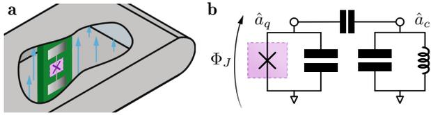
**Fig. 2 Quantizing a simple circuit.** **a** Illustration of a 3D cavity enclosing a transmon qubit chip. The cross symbol marks the location of a Josephson junction. Vertical blue arrows depict the electric field  $\vec{E}_m(\vec{r})$  of the fundamental cavity mode, TE<sub>101</sub>. **b** Equivalent two-mode lumped-element representation of the distributed circuit. Operators  $\hat{a}_q$  and  $\hat{a}_c$  denote the qubit and cavity mode operators, respectively.
