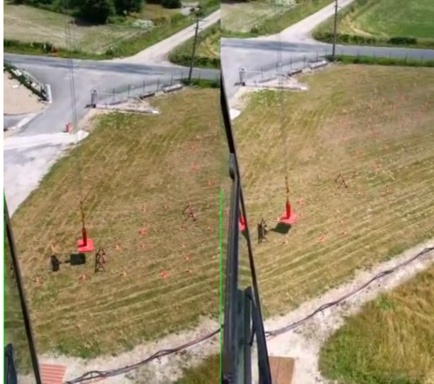
Figure 8: The “hurdle course” set in place to compare performances with (right picture) and without (left) the open-loop automated assistance, viewed from the operator’s cabin. The crane is 40 meters high and the load weighs one ton. It took the operator 75 seconds to go past the two hurdles with the assistance on, whereas it took 110 seconds without it. Image courtesy of Manitowoc.
