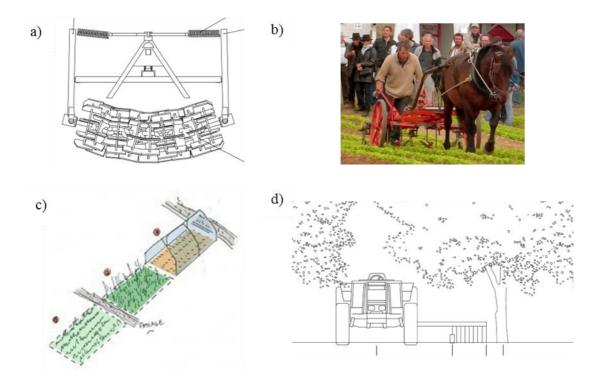
Figure 2. Pictures and drawings presenting implements appropriate to particular situations: a) a Rolofex; b) a Neo bucher; c) a movable greenhouse; and d) a Sandwich tillage implement (from https://www.latelierpaysan.org/)
