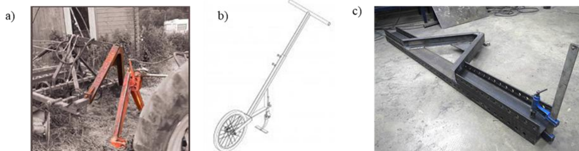
295 296 Figure 3. Pictures and drawings presenting adaptable implements: a) a quick hitch triangle; b) a 297 market gardening hoe; and c) a tractor tool bar (from https://www.latelierpaysan.org/ )
