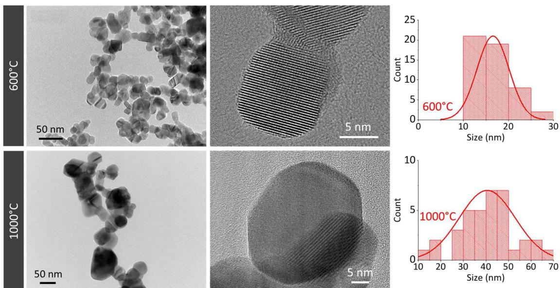
**Figure 7:** TEM images and particles size distribution of SnO<sub>2</sub> nanoparticles prepared by sol-gel method and heat-treated at two different temperatures.
