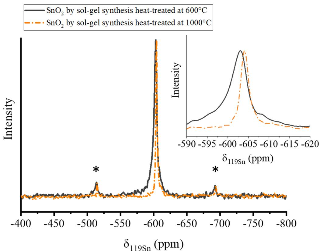
**Figure 8:**  $^{119}\text{Sn}$  solid-state NMR spectra of  $\text{SnO}_2$  obtained by sol-gel syntheses heat-treated at  $600^\circ\text{C}$  and  $1000^\circ\text{C}$ , with spinning sidebands denoted \*.
