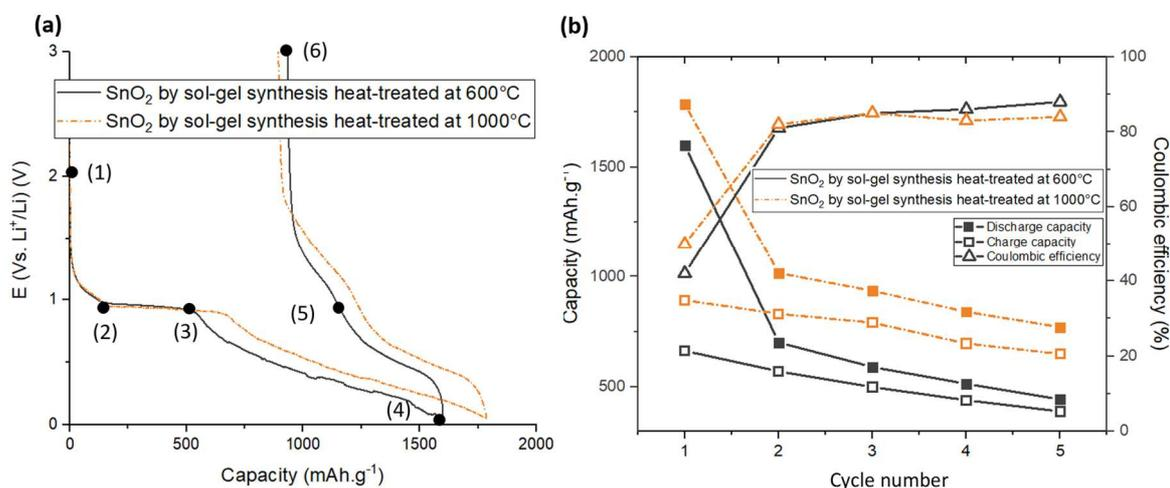
**Figure 9 :** (a) First Discharge/Charge curve at 10 mA.g<sup>-1</sup> of SnO<sub>2</sub> obtained by sol-gel synthesis particles heat-treated at 600°C and 1000°C. (b) Comparison of cycling performance and coulombic efficiency of the materials at 10 mA.g<sup>-1</sup>.
