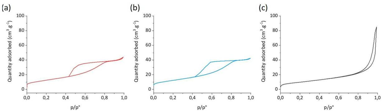
**Figure 3:** 77K N<sub>2</sub> isotherms of (a) solvothermal, (b) hydrothermal and (c) sol-gel syntheses.
