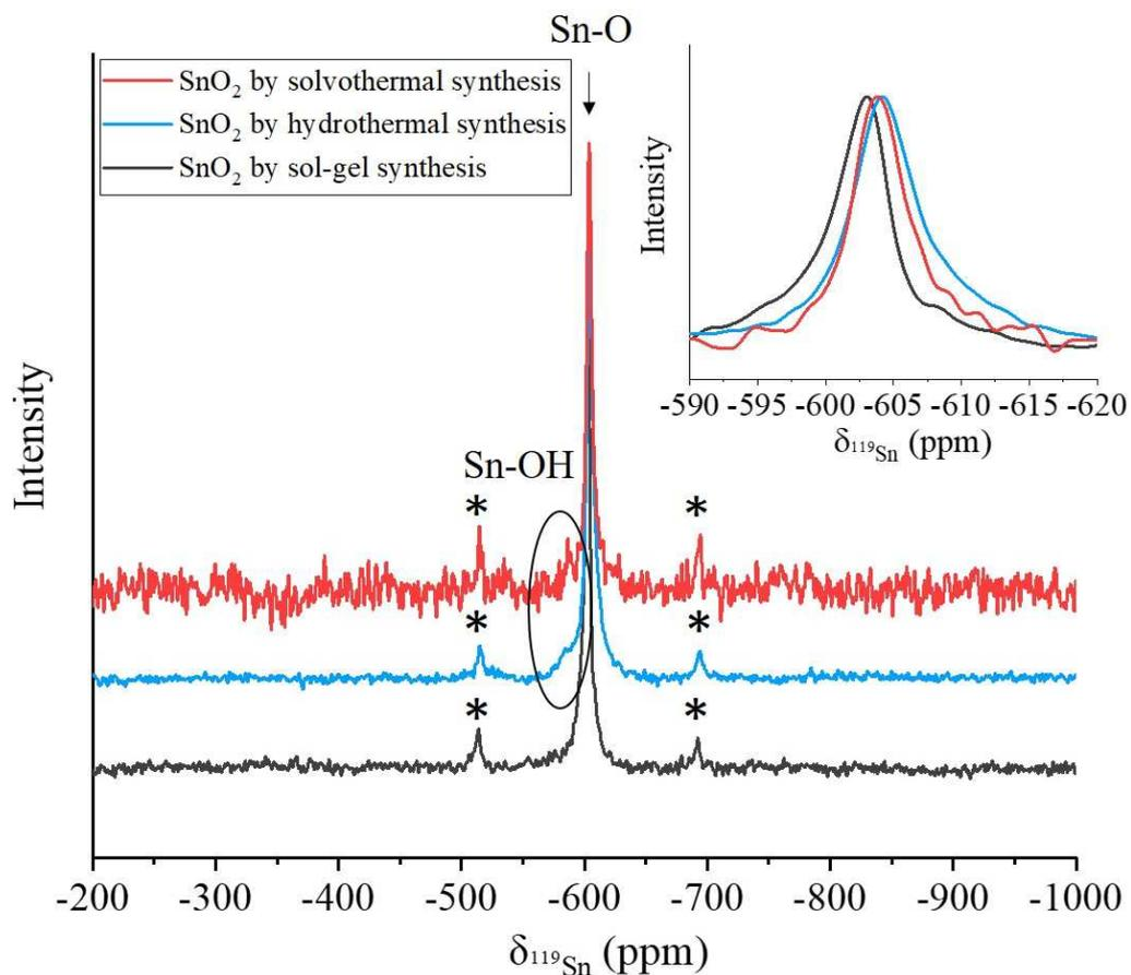
**Figure 5 :** <sup>119</sup>Sn solid-state NMR spectra of solvothermal, hydrothermal and sol-gel SnO<sub>2</sub>, with spinning sidebands denoted \*.
