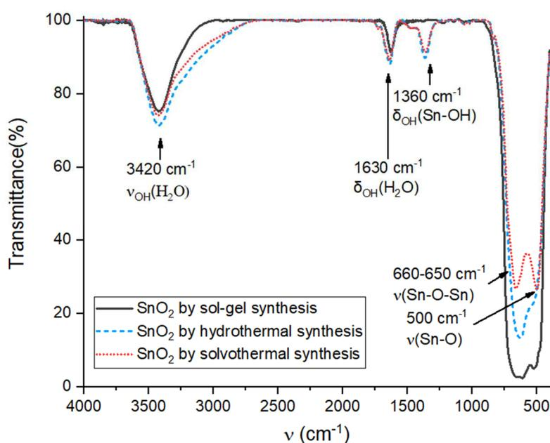
**Figure 4 :** Infrared spectra of spectra of solvothermal, hydrothermal and sol-gel SnO<sub>2</sub> materials
