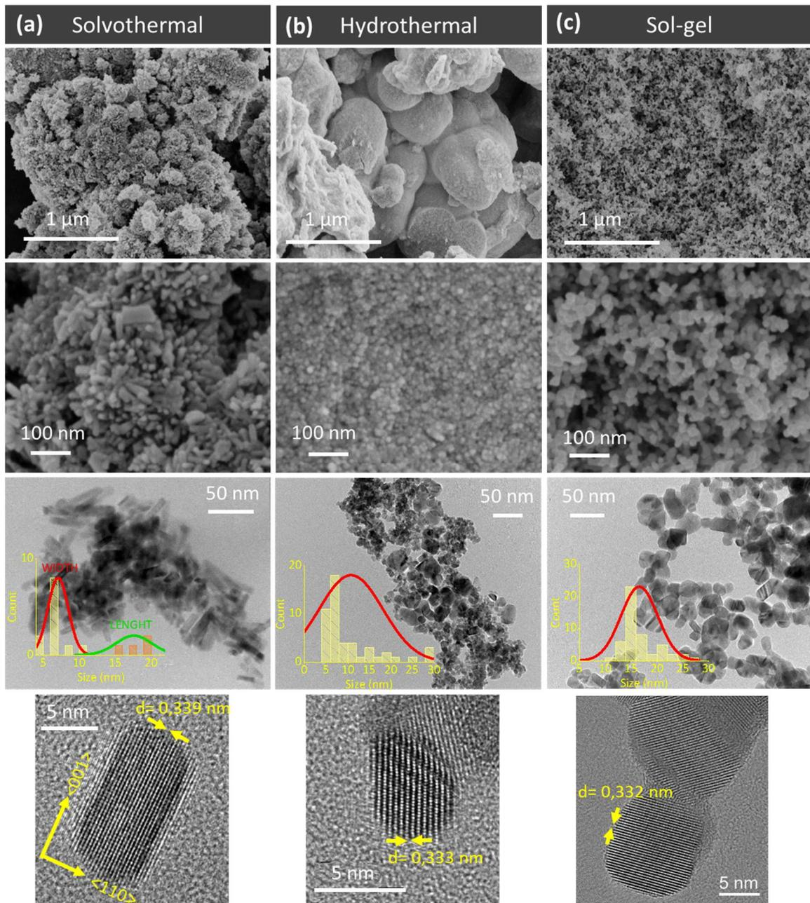
**Figure 2 :** SEM and TEM images and particles size distribution of SnO<sub>2</sub> nanoparticles prepared by
