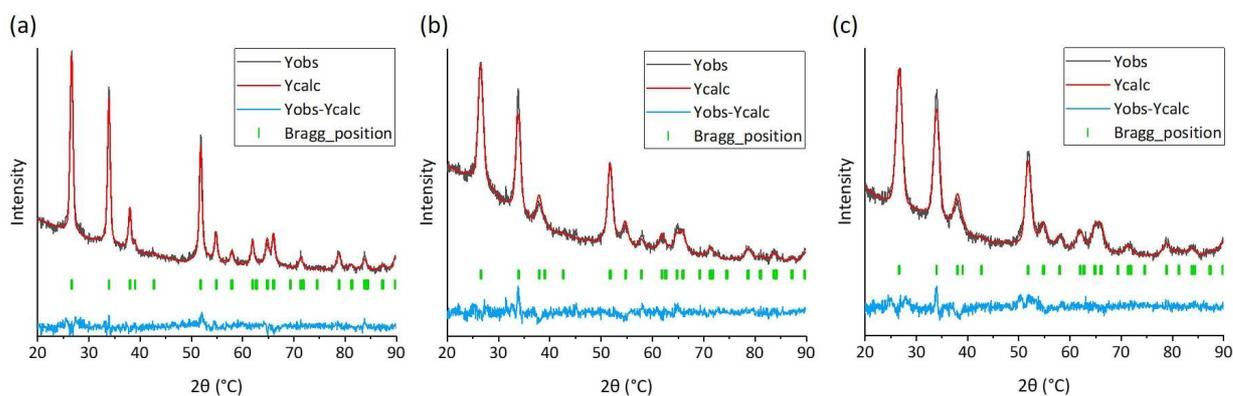
**Figure 1 :** XRD powder pattern profiles and Le Bail refinements of SnO<sub>2</sub> nanoparticles obtained by (a) sol-gel, (b) hydrothermal and (c) solvothermal syntheses.
