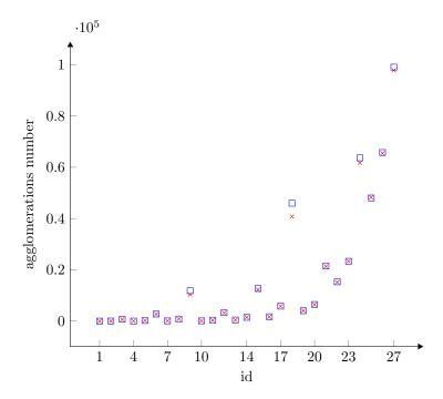
Figure B.10: Results (values in table B.3) in terms of agglomerations number during the time-step  $\Delta t=1\,\mathrm{s}$  for mean field calculations (red cross) (equations A.1, A.2, A.15 and A.16) and full field simulations (blue squares) (200 000 spheres placed without superposition inside a cube).
