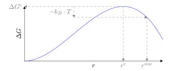
Figure 2: Free enthalpy change  $\Delta G$  induced by forming a spherical precipitate as a function of its radius r. Critical radius  $r^c$ , nucleation radius  $r^{\text{nuc}}$  and free enthalpy barrier  $\Delta G^c$ .
