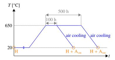
Figure 4: Thermal treatments to trigger the  $\gamma''$  precipitation. Material states as-received *i.e.* homogenized (H) then annealed at 650 °C for 100 h (H + A<sub>100</sub>) and 500 h (H + A<sub>500</sub>).
