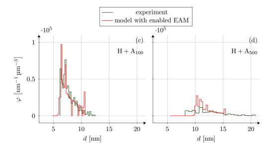
Figure 6: Number density distributions  $(\varphi)$  of the equivalent diameter (d) of the  $\gamma''$  precipitates, normalized per unit volume of material, experimental (green) and calculated by the model (red) after (a,c) 100 h (H + A\_{100}) and (b,d) 500 h (H + A\_{500}) at 650 °C when enabling (a,b) (pagg = 5) and disabling (c,d) (pagg = 0) the EAM.
