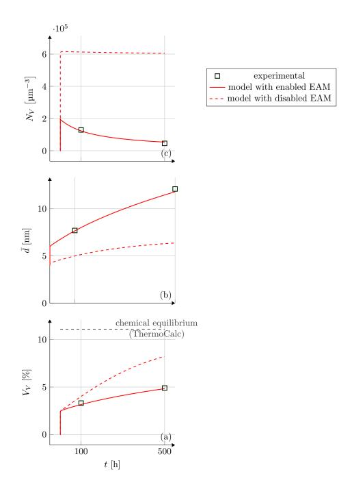
Figure 7: (a) number  $(N_V)$  per unit volume, (b) mean equivalent diameter  $(\bar{d})$  and (c) Volume fraction  $(V_V)$  of precipitates over time, experimental (squares) and calculated by the model (lines). Continuous and dashed lines correspond to the enabled and disabled equivalent agglomeration model (EAM), respectively.
