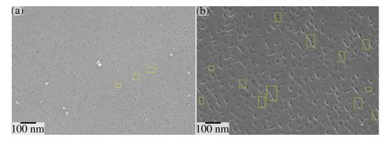
Figure 5: Agglomerating or about-to-agglomerate  $\gamma''$  precipitates (yellow rectangles) in material states (a) H + A<sub>100</sub> and (b) H + A<sub>500</sub>.
