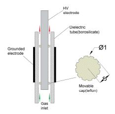
Scheme 2. Schematic diagram of the DBD reactor.
