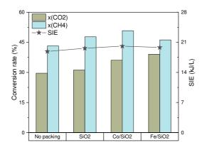
Figure 3. The conversion rates and SIE of the experiments without packing, with SiO<sub>2</sub> only, and with catalysts (peak-to-peak voltage: 5.5 kV, frequency: 3 kHz, total flow rate: 30 mL/min,  $CO_2/CH_4$  ratio = 2:1).
