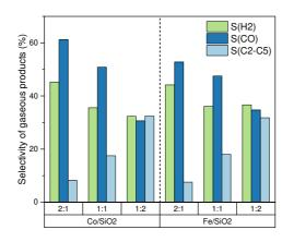
Figure 8. The selectivity of gaseous products as a function of catalysts and a  $CO_2/CH_4$  ratio from 2:1 to 1:2 (peak-to-peak voltage: 5.5 kV, frequency: 3 kHz, total flow rate: 30 mL/min).
