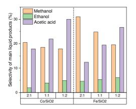
Figure 7. The selectivity of main liquid products as a function of catalysts and a  $CO_2/CH_4$  ratio from 2:1 to 1:2 (peak-to-peak voltage: 5.5 kV, frequency: 3 kHz, total flow rate: 30 mL/min).
