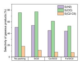
Figure 5. The selectivity of gaseous products without packing, with  $SiO_2$  only, and with catalysts (peak-to-peak voltage: 5.5 kV, frequency: 3 kHz, total flow rate: 30 mL/min,  $CO_2/CH_4$  ratio = 2:1).
