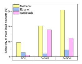
Figure 6. The selectivity of main liquid products without packing, with SiO<sub>2</sub> only, and with catalysts (peak-to-peak voltage: 5.5 kV, frequency: 3 kHz, total flow rate: 30 mL/min, CO<sub>2</sub>/CH<sub>4</sub> ratio = 2:1).
