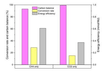
Figure 2. The carbon balance, conversion rates, and energy efficiency of CH<sub>4</sub>-only or CO<sub>2</sub>-only conditions without catalysts (peak-to-peak voltage: 5.5 kV, frequency: 3 kHz).
