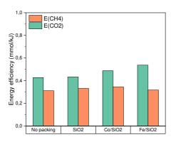
Figure 4. The energy efficiency of  $CO_2$  and  $CH_4$  without packing, with  $SiO_2$  only, and with catalysts (peak-to-peak voltage: 5.5 kV, frequency: 3 kHz, total flow rate: 30 mL/min,  $CO_2/CH_4$  ratio = 2:1).
