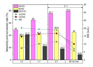
Figure 1. The selectivity of gaseous products, the conversion rates of reactants and the corresponding SIE varied by  $CO_2/CH_4$  ratio and total flow rate without catalysts (peak-to-peak voltage: 5.5 kV, frequency: 3 kHz).
