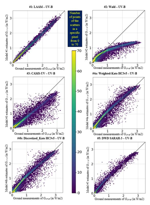
Fig. 3: 2-D histograms of the UV-B derived from the 6 different models (vertical axes) and UV-B in-situ measurements (horizontal axis). Models are respectively: #1 LAAM, #2 Wald, #3 CAMS-UV, #4a Weighted\_Kato HC3v5, #4b Discretized\_Kato HC3v5, and #5 DWD SARAH-3
