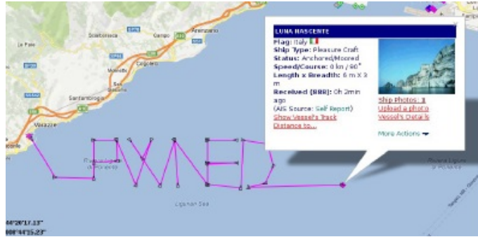
Figure 1: Example of a spoofed ship following a programmed path, from Balduzzi et al. (2014a) (in print, colour should be used for this Figure)
