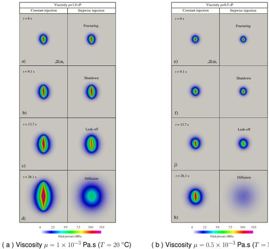
Figure 8: Fluid driven fracture patterns and diffused fluid pressure contours for the two schemes of injection and for low different values of fluid viscosity, i.e.  $\mu = 1 \times 10^{-3}$  Pa.s corresponding to  $T = 20$  °C and  $\mu = 0.5 \times 10^{-3}$  Pa.s corresponding to  $T = 55$  °C. These contours and fracture patterns are plotted for several injection times which correspond to the letters (a to h) in Fig. 7.
