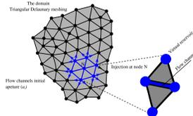
Figure 2: Conceptual graph that illustrates the implementation of fluid diffusion and leak-off in the FDEM approach.
