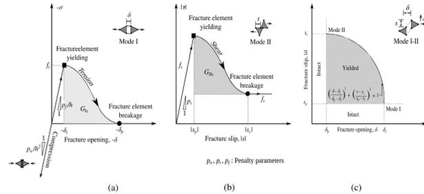
Figure 1: Penalty coefficients and fracture energies for different modes of fracturing adopted in FDEM [1].
