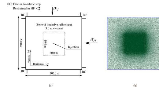
Figure 6: (a) The geometry and boundary conditions of domain chosen for the HF simulations (Irazu code).
