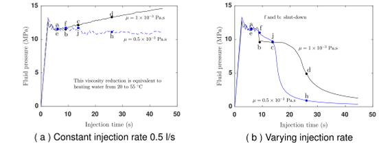
Figure 7: Net fluid pressure profile due to injection a) at constant rate of 0.5 l/s, b) at constant rate of 0.5 l/s for the first 9.1 s and then shutting down.
