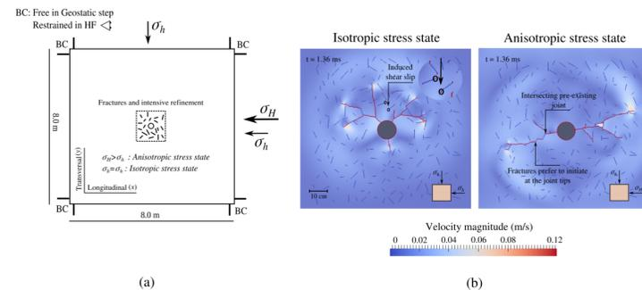
Figure 3: a) The model of the simulations used in the Y-Geo code. b) Fracture patterns for the cases of isotropic and anisotropic stress states in a heavily fractured rock formation at time of 1.36 ms since injection. The trajectories are plotted in the field of velocity magnitude.
