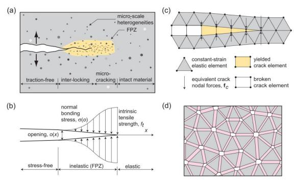
**Figure 1.** Material failure modelling in FDEM. (a) Conceptual model of a tensile crack in a heterogeneous rock material. (b) Theoretical FPZ model. (c) FDEM implementation of the FPZ using triangular elastic elements and four-noded crack elements to represent the bulk material and the fracture, respectively. (d) FDEM representation of a fracturable body with continuum triangular elements and embedded crack elements indicated in grey and pink, respectively.
