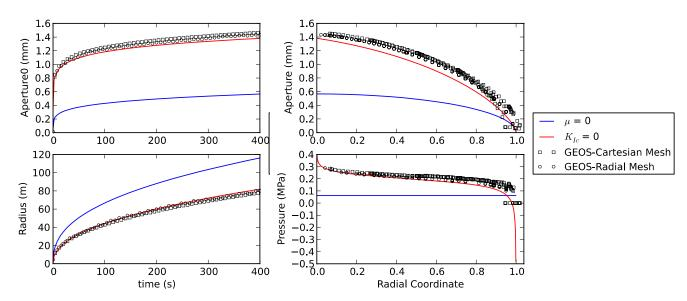
**Figure 3.** Comparison of GEOS against asymptotic solutions for viscosity dominated case, (Savitski and Detournay, [2002]). Fracture radius and wellbore aperture are plotted versus time, and the aperture and pressure profiles at the end of the simulation are plotted against the radial coordinate.
