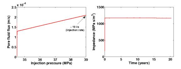
Figure 5: (left) Relation between injected pore fluid pressure and created fluid flux at the injection well GPK1 of unenhanced HDR reservoir at Soultz-sous-Forêts. The fluid flux increases linearly following the injection schedule shown on figure 2(right); (right) Impedance profile: an impedance greater than 1000 MPa/(m<sup>3</sup>/s) indicates inefficient operation.
