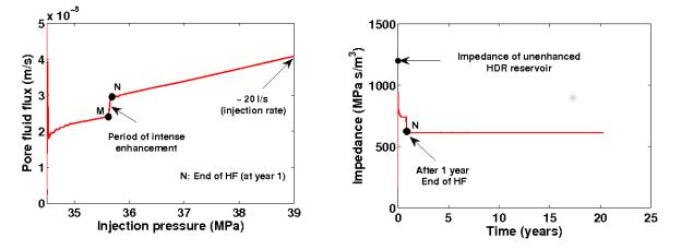
Figure 11: (left) Relation between injected pore fluid pressure and fluid flux at the injection well GPK1: non-linear relation results from the creation of improved connections; (right) Impedance profile of the enhanced HDR reservoir.
