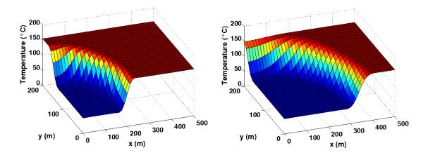
Figure 4: Contours of the temperature of the reservoir at year 5 (left) and year 10 (right); simulations without HF.
