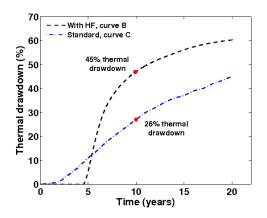
Figure 13: Thermal drawdown of the mean production temperature for the enhanced HDR reservoir curve B, and the standard production temperature as suggested by Kolditz [1995].
