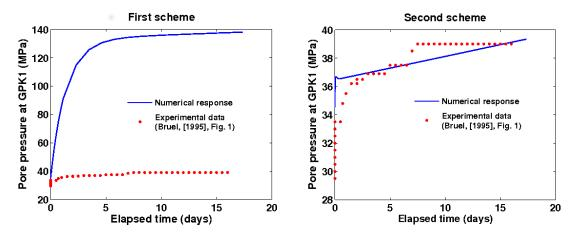
Figure 3: Injection pressure at GPK1 during the 1993 field injection test at Soultz-sous-Forêts: (left) impermeable boundaries; (right): permeable boundaries. Comparison between experimental data and the HFM responses for the two schemes sketched on Table 3.
