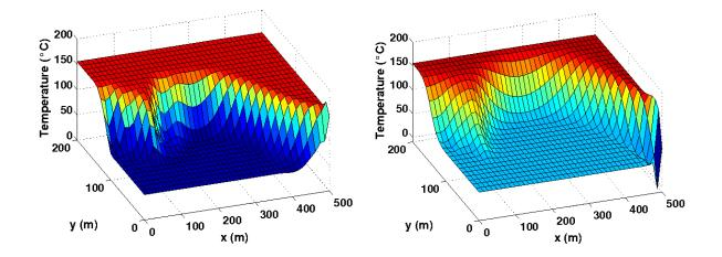
Figure 7: Contours of the reservoir temperature at year 5 (left) and year 10 (right); HF model is activated. Convection of heat is dominant in the direction of fracture evolution.
