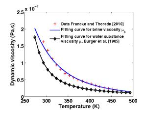
Figure 14: Viscosities of water and brine containing 0.225 kg of NaCl per kg of solution as a function of temperature at a constant pressure of 1.5 MPa.
