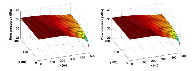
Figure 8: Contours of the reservoir pressure at year 5 (left) and year 10 (right); HF model is activated. The high permeability created by HF levels the pressure contours in the region of enhancement.
