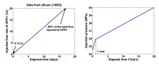
Figure 2: Injection conditions at GPK1 during the 1993 field injection test at Soultz-sous-Forêts (left) linear injection flow rate at early times, (right) time course of injection pressure at later times. The actual test includes injection at GPK1 well and production at two wells which are considered to be located symmetrically with respect to GPK1. Only a quarter of the reservoir is meshed.
