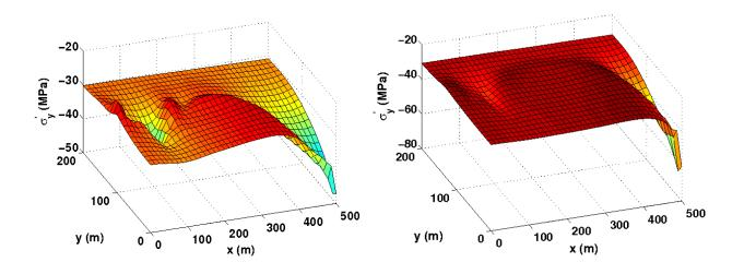
Figure 10: Contours of transversal effective stress  $\sigma'_{vv}$  at year 5 (left) and year 10 (right); HF model is activated.
