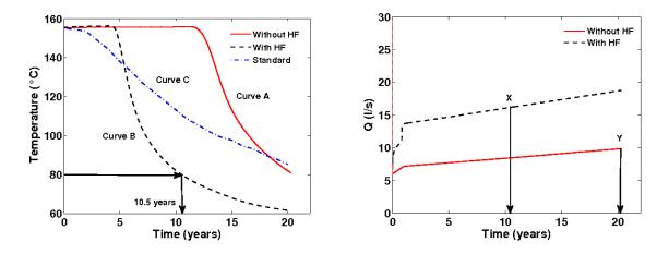
Figure 12: (left) Profiles of produced fluid temperature with HF and without HF; (right) Produced flow rate from the enhanced reservoir is two-fold the produced flow from the natural reservoir.
