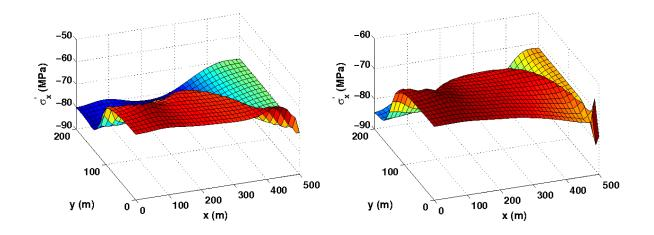
Figure 9: Contours of longitudinal effective stress  $\sigma'_{xx}$  at year 5 (left) and year 10 (right); HF model is activated. Stresses are dawdled in compression in the cooled regions due to tensile stresses.
