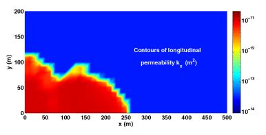
Figure 6: Contours of longitudinal permeability component k<sub>xx</sub> (m<sup>2</sup>) at year 1 of pumping; HF model is activated.
