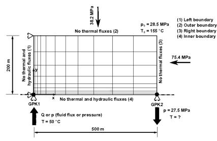
Figure 1: Mesh in the horizontal plane (x, y), initial and boundary conditions used for the stimulation tests at the Soultz-sous-Forêts HDR reservoir, *figure is not to scale*.
