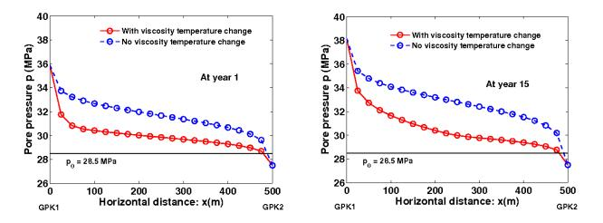
Figure 15: Pore pressure profiles along the line joining the injection and production wells, at year 1 and year 15. Solid lines: temperature-dependent viscosity; dashed lines: constant brine viscosity  $\mu_b = 3 \times 10^{-4} \text{ Pa} \times \text{s}$ .
