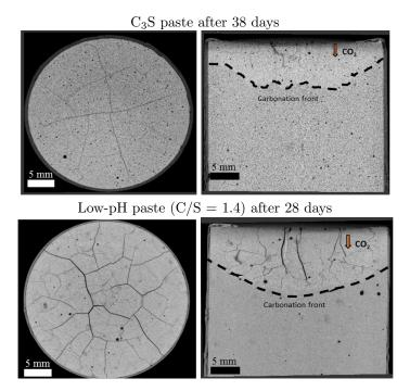
Figure 2:  $\mu$ CT scan of samples subjected to accelerated carbonation (voxel size = 17  $\mu$ m). Left panel: top view of the sample, right panel: transverse view of the sample. These scans show the evolution of the carbonation front as well as the appearance of cracks. Measurement of the extent of the carbonation front were coupled with XRD profiles, thermogravimetric analysis and phenolphtaleine tests.
