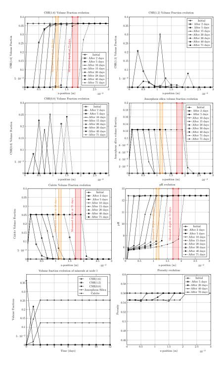
Figure 8: Evolution of the mineralogical and pH profiles during the accelerated carbonation of the low-pH paste. Measured carbonation dephs after 28 and 71 days (given in table 2) are highlighted in orange and red. 19
