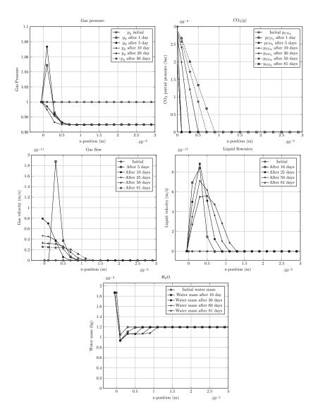
Figure 5: Evolution of gas and liquid flow parameters during the accelerated carbonation.
