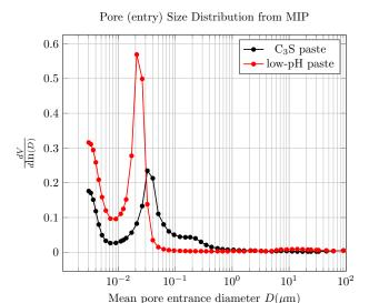
Figure 1: Representation of the pore size distributions of the two samples obtained by MIP, indicating a finer porosity for the low-pH paste.
