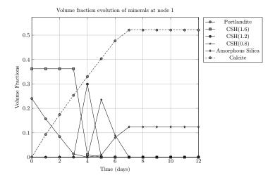
Figure 4: Evolution of mineralogy in the first two milimeters of the  $C_3S$  paste over time
